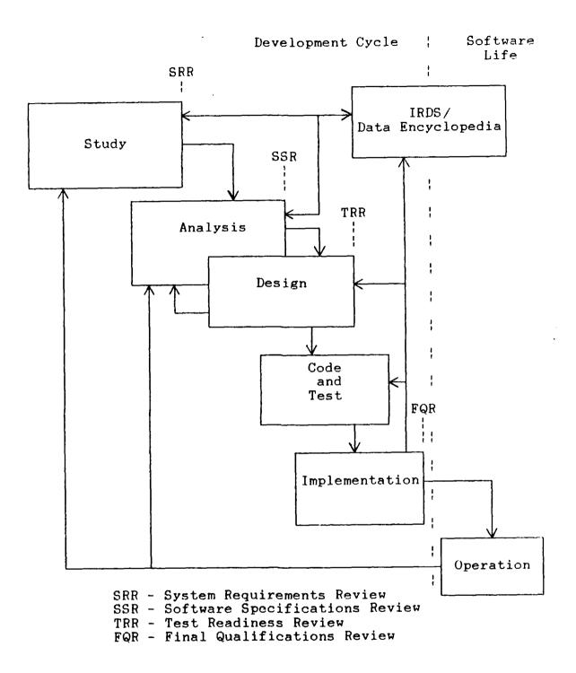
Figure 4-1. Proposed DoD STD-2167A Life Cycle Using CASE
