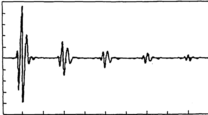
Figure 1. First five back-surface echoes received from an 0.5-inch-thick aluminum plate. Linear amplitude scale (arbitrary values) versus horizontal time scale of 2.048 microseconds per division extending from 3 to 23.48 microseconds.
