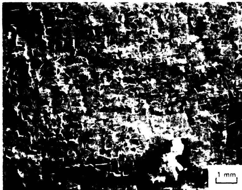
Figure 14. SEM micrograph shows a characteristic mosaic crack pattern on the fracture surface of the composite specimen with 6-mil-thick PEI film adhesive.
