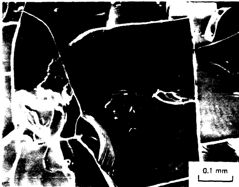
Figure 16. SEM micrograph shows nucleation point and growth band markings on the composite fracture surface.
