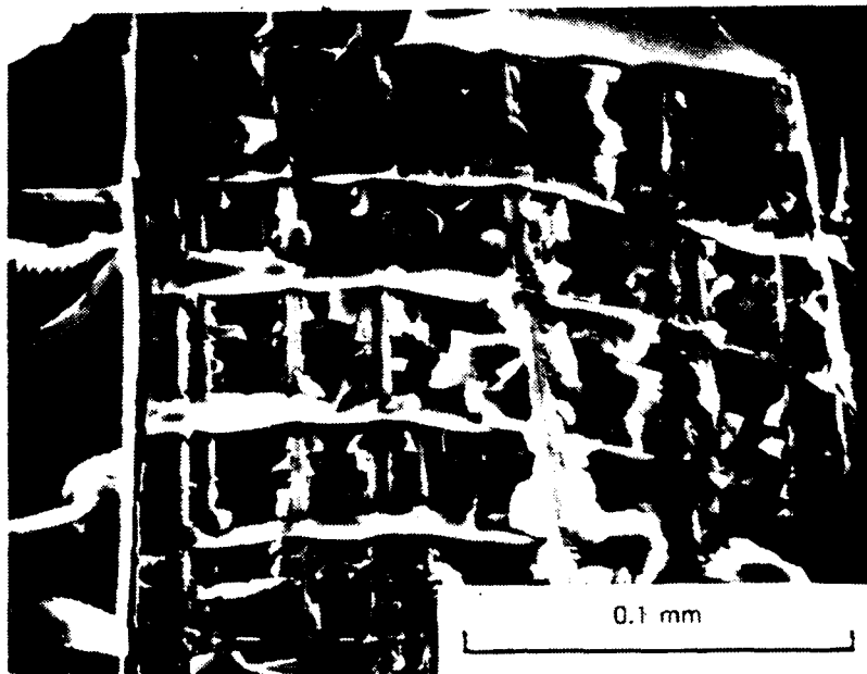
Figure 10. SEM micrograph shows matrix cracks perpendicular to the fibers on the fractured composite specimen.
