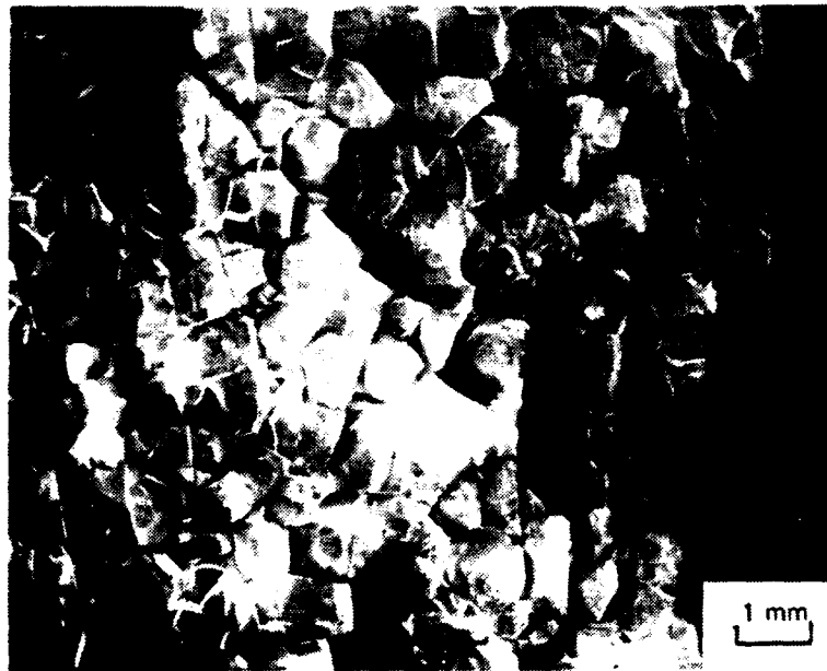
Figure 13. SEM micrograph shows a characteristic mosaic crack pattern on the fracture surface of the composite specimen with 18-mil-thick PEI film adhesive.
