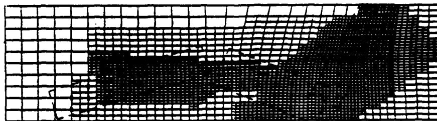
Figure 5. Grids created for the adaptive mesh solution at t = .038, 0.076, 0.114, 0.152, and 0.19 (top to bottom). The rectangular boxes represent the error clusters used to move the mesh for the current time step.
