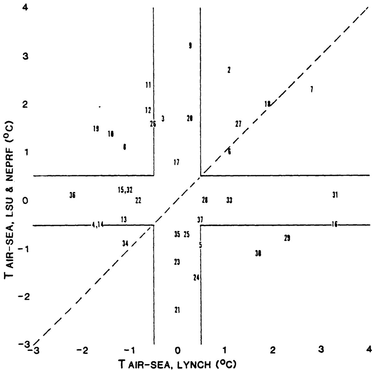
Figure 2. USNS LYNCH air-sea temperature differences: abscissa, LYNCH crew; and ordinate, LSU & NEPRF. Data are given by radiosonde launch sequence number. Dashed line represents perfect correlation. Neutral stability,  $T_{\text{air-sea}} \leq 0.5^{\circ}\text{C}$ , delineated for each data set.
