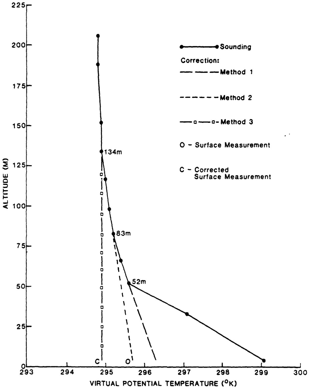
Figure 1. USNS LYNCH sounding of 28 June 1149 GMT, with Method 1, 2, 3 profile corrections.
