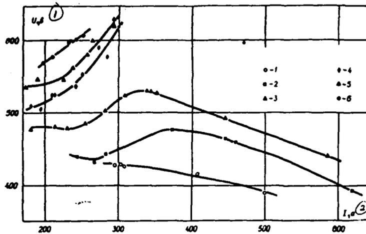
Figure 3. Volt-ampere characteristics of the arc at different flow rates of gas ( $G_r$ ): 1 - 14, 2 - 17, 3 - 19, 4 - 25, 5 - 30, 6 - 35 g/s. Flow rate of protective gas ( $G_p$ ) - 3 g/s. Working section of anode - 40 mm.
