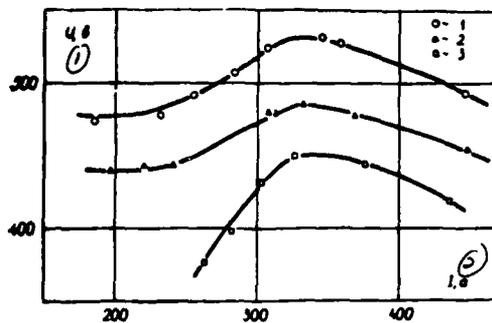
Figure 4. Volt-ampere characteristics of the arc depending on the kind of protective gas.  $G_r$  - 19,  $G_p$  - 2 g/s. 1 - protective gas - (N<sub>2</sub>), 2 - without protective gas, 3 - protective gas - (Ar).
