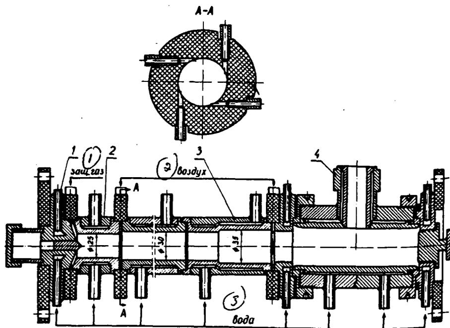
Figure 2. Vortex-type dc electric-arc heater. 1 - cathode; 2 - interelectrode insert; 3 - multistage anode; 4 - mixing chamber.
