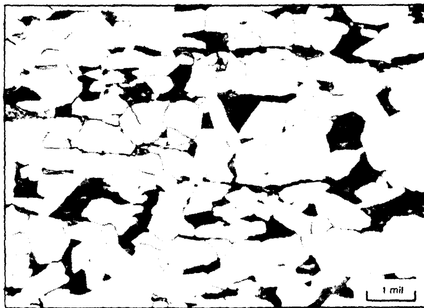
Figure 5. Microstructure of provision material, Nital etch. Banding can be seen in microstructure. Dark regions are pearlite.
