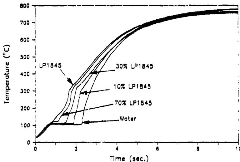
Fig. 4. The thermal traces of H<sub>2</sub>O and LPG1845 and H<sub>2</sub>O dilutions of LPG1845 all heated at an initial rate of about 150°C s<sup>-1</sup> under 15 psi Ar.
