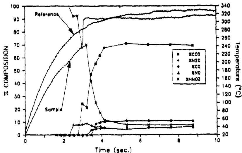
Fig. 7. The relative concentrations of the IR active gas products (excluding  $H_2O$ ) when  $1.5 \mu L$  of LPG1845 is heated at  $dT/dt = 110^\circ C s^{-1}$  under 500 psi Ar. The reference and sample thermal traces are superposed.
