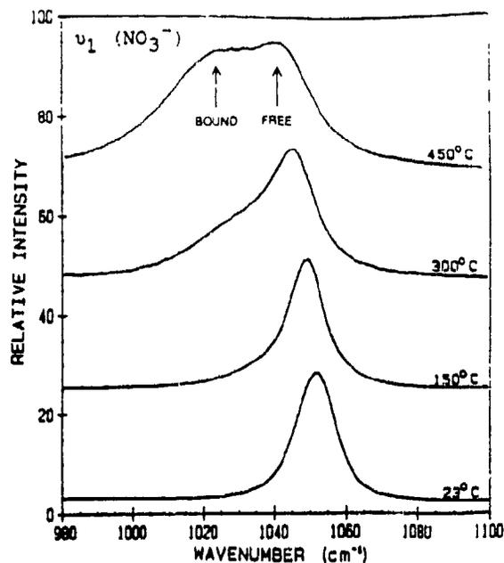
FIG. 6. The temperature dependence of the  $\nu_1(NO_3^-)$  symmetric stretch, showing the increased contact-ion pairing of aqueous  $Zn(NO_3)_2$  as the temperature is raised.
