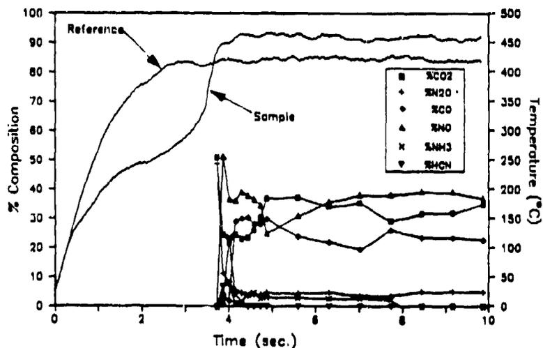
Fig. 3. The IR active gas products evolved from solid TEAN under 200 psi Ar with  $dT/dt = 175^\circ C s^{-1}$ . The filament reference trace and the thermal trace with 3 mg of TEAN are shown.
