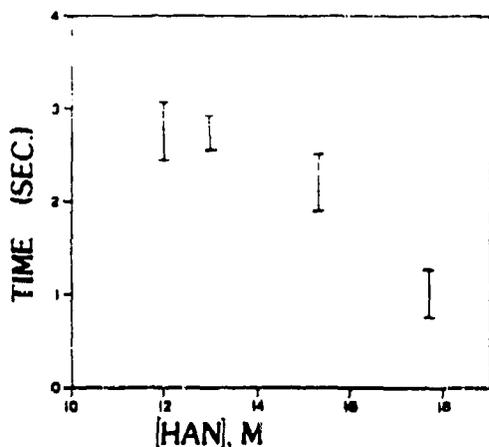
Figure 5. The relationship of the initial  $[\text{HNO}_3] = [\text{N}_2\text{O}]$  crossover (see Figure 4) to the  $\text{H}_2\text{O}$  content of the HAN sample ( $dT/dt = 130 \text{ K s}^{-1}$ ,  $T_f = 510 \text{ K}$ ,  $P = 500 \text{ psi}$  of Ar). Damp solid HAN was estimated to be 17.5 M.
