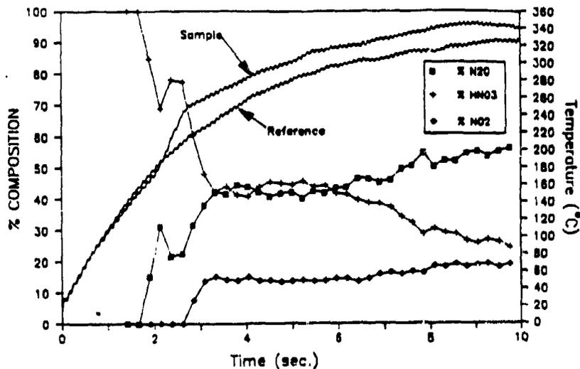
Fig. 2. The IR active gas products (excluding  $H_2O$ ) evolved from the thermolysis of solid HAN at  $dT/dt = 80^\circ C s^{-1}$  under 200 psi Ar. Overlaid on these products is the thermal trace of the bare filament and the thermal trace of the filament with 2.5 mg of solid HAN spread evenly on it.
