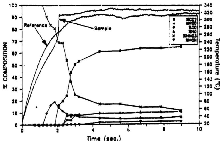
Fig. 8. The relative concentrations of the IR active gas products (excluding  $H_2O$ ) when  $1.5 \mu L$  of LGP1845 is heated at  $dT/dt = 120^\circ C s^{-1}$  under 1000 psi Ar. The reference and sample thermal traces are superimposed.
