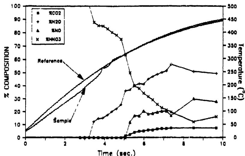
Fig. 5. The relative concentrations of the IR active gas products (excluding  $\text{H}_2\text{O}$ ) when  $2.0 \mu\text{L}$  of LGP1845 is heated at  $dT/dt = 70^\circ\text{C s}^{-1}$  under 15 psi Ar. The reference and sample thermal traces are superimposed on these data.
