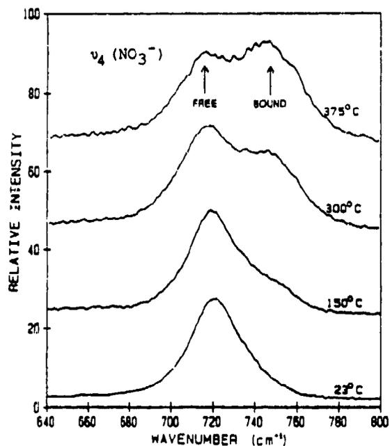
FIG. 5. The temperature dependence of the  $\nu_4(NO_3^-)$  in plane bending mode, showing the increased amount  $Zn^{2+}-ONO_2^-$  of contact-ion pairing at higher temperature.
