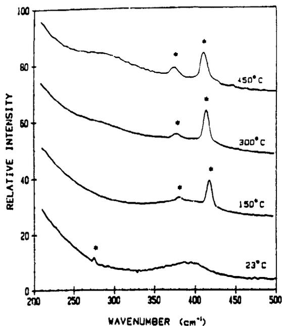
FIG. 4. The  $Zn(H_2O)_6^{2+}$  region ( $\sim 385\text{ cm}^{-1}$ ) and  $Zn^{2+}-ONO_2^-$  stretch ( $\sim 292\text{ cm}^{-1}$ ) as a function of temperature. The starred absorptions result from sapphire.
