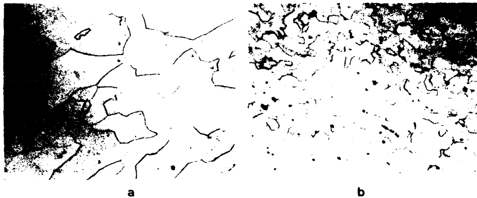
Fig. 8. Microscopic inclusions of foreign material of a few \mu\text{m} diameter for material of a) high and b) low purity. Inclusions were made visible by etching the mechanically polished Nb samples.
