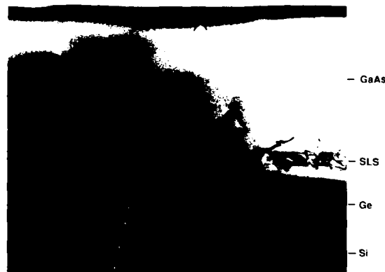
Fig. 8. Transmission electron micrograph of a GaAs/GaAs-GaAsP SLS structure grown on Ge/Si composite substrate. The GaAs layer is 2 \mu\text{m} thick. The germanium film on silicon was grown by MBE, the GaAs and GaAsP were grown by MOCVD. [Adapted from (20)]
