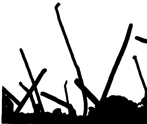
Fig. 4. A shadowgraph of whiskers from an accelerated pressure tested matte tin deposit. 850X.
