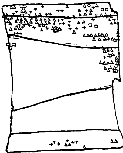
C) Composite of fracture pattern at 30% deformation, 5.25 \times 10^{-3} m/min.
