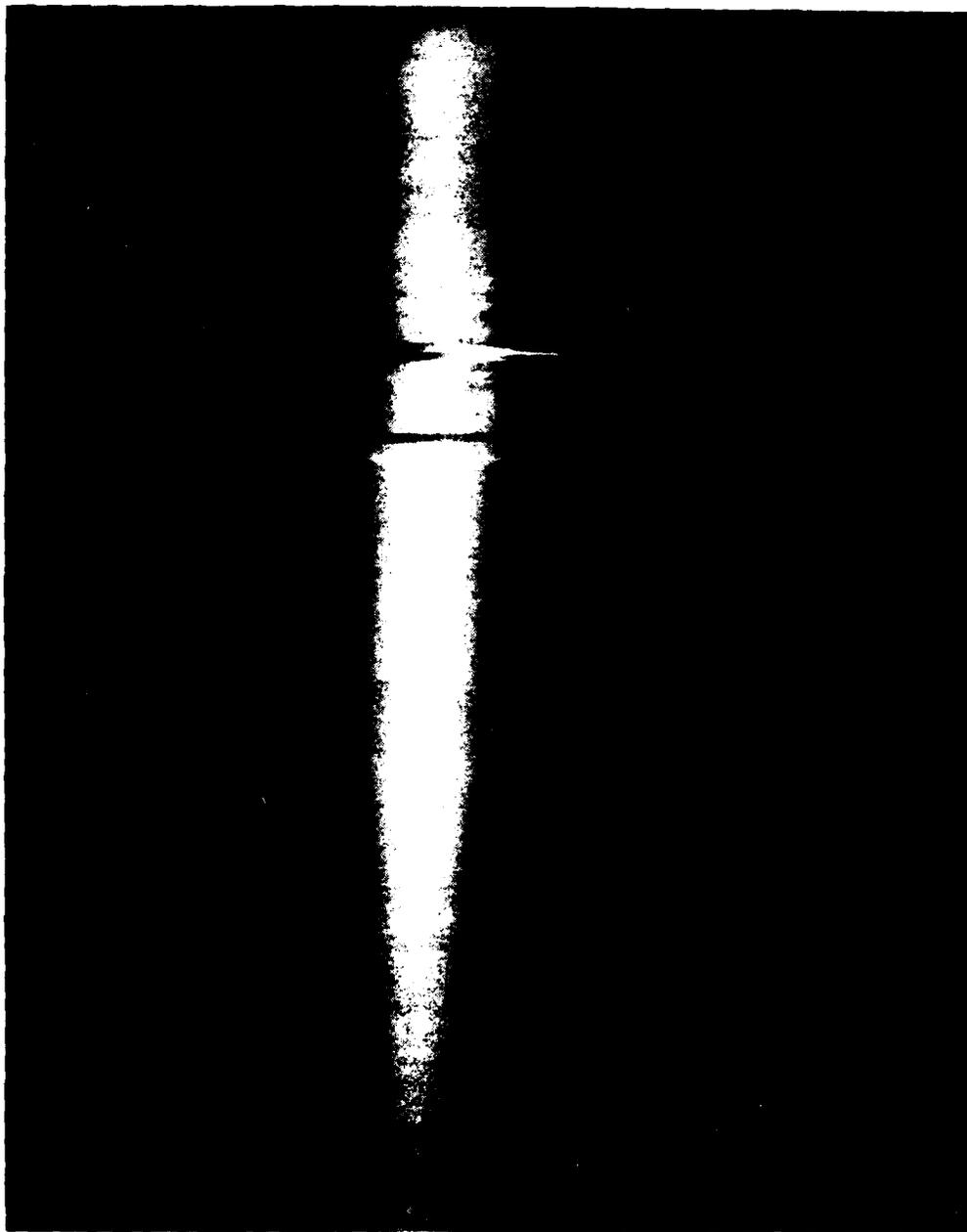
Figure 4. Photograph of flowing argon afterglow with no grids in the flow tube.
