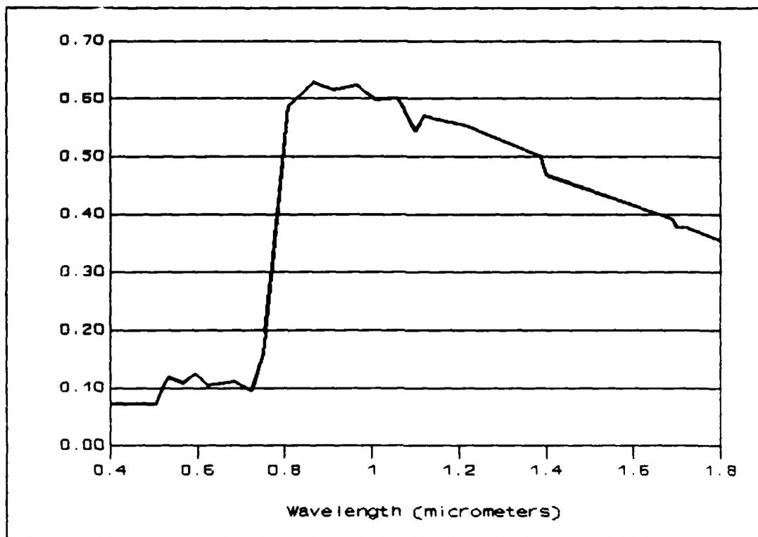
Figure D1. Reflectance of US Army Olive Drab vs Wavelength (IPRC:569)
