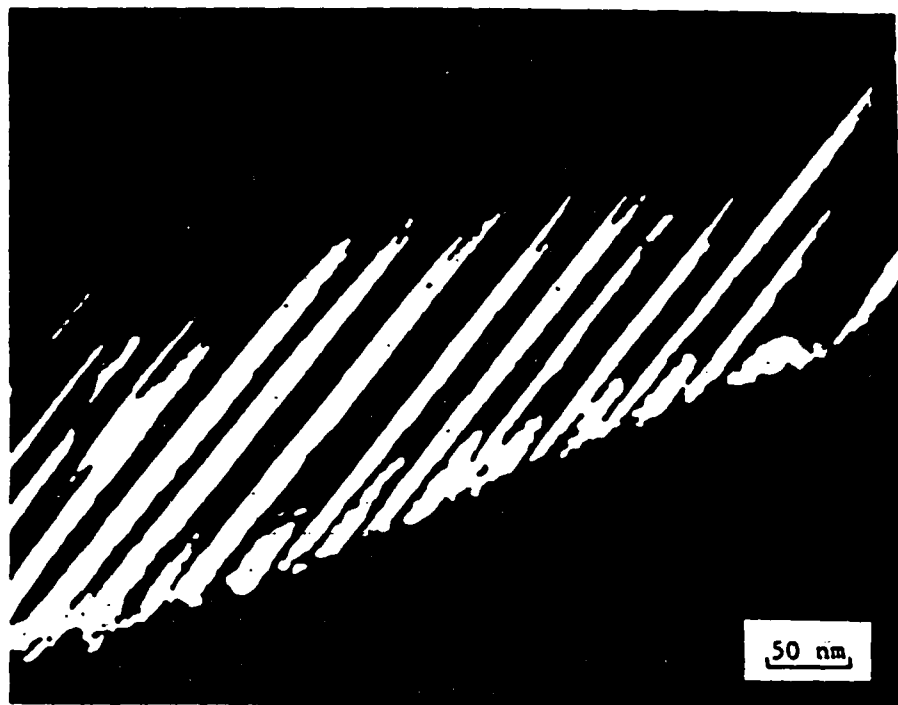
Fig. 6. Dark field TEM micrograph of YBa 2 Cu 3 O 7-x showing twinning.
