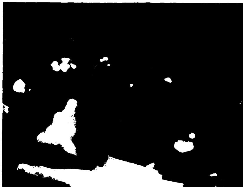
FIGURE 25. Cu "RICH" PARTICLES ATTACHED TO SiC WHISKERS AT THE BOTTOM OF A PIT ON SiC/AA-2124-T6M (10K X)
