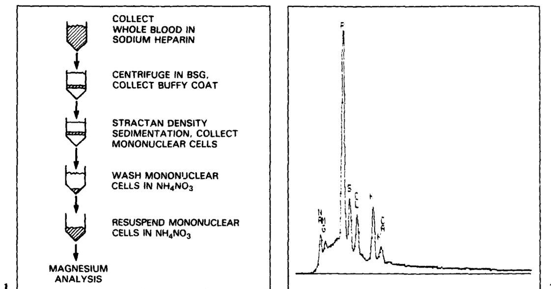
Fig. 1. The Stractan MBC isolation method is diagrammed.
