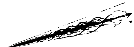
Fig. 2. Hydrogen bubble-wire visualization of leading edge vortex flow for conditions below the critical angle of attack.
