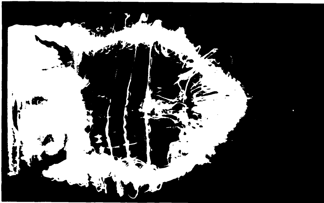
Fig. 10 Nikon shot of vortex system of a rectangular wing with aspect ratio 2 after a rapid pitch from 0^\circ to 60^\circ ; c = 15.2 cm, U_\infty = 61 cm/sec.
