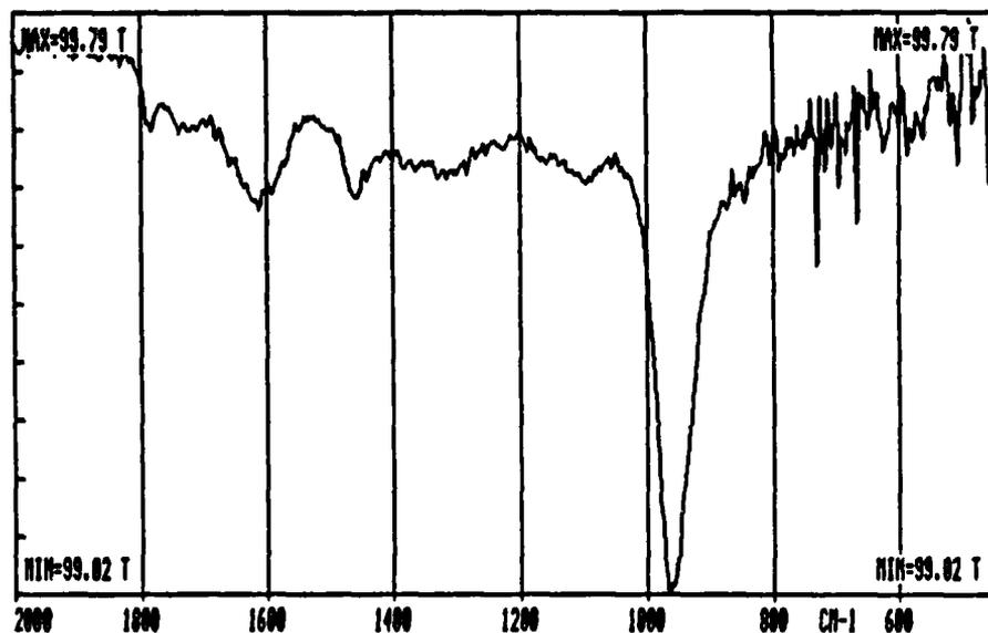
Figure 8. RAIR spectrum obtained from a thin film of NMA that was applied to a polished 2024 aluminum mirror, heated for two hours at 150°C, and then rinsed with acetone.
