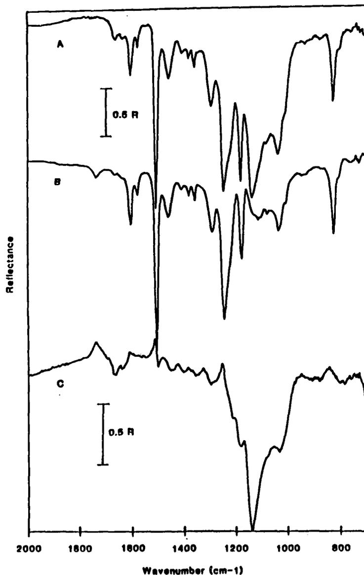
Figure 3. RAIR spectra of (A) - the failure surface of a DCB prepared from a steel substrate primed with  $\gamma$ -APS and an epoxy cured with a tertiary amine curing agent, (B) - a film of the same epoxy deposited on a polished steel substrate, and (C) - the difference of A and B. In A and B the epoxy was cured at 150°C for one hour.
