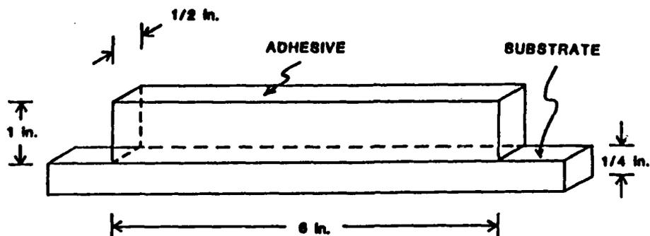
Figure 1. Double cantilever beam test specimen.
