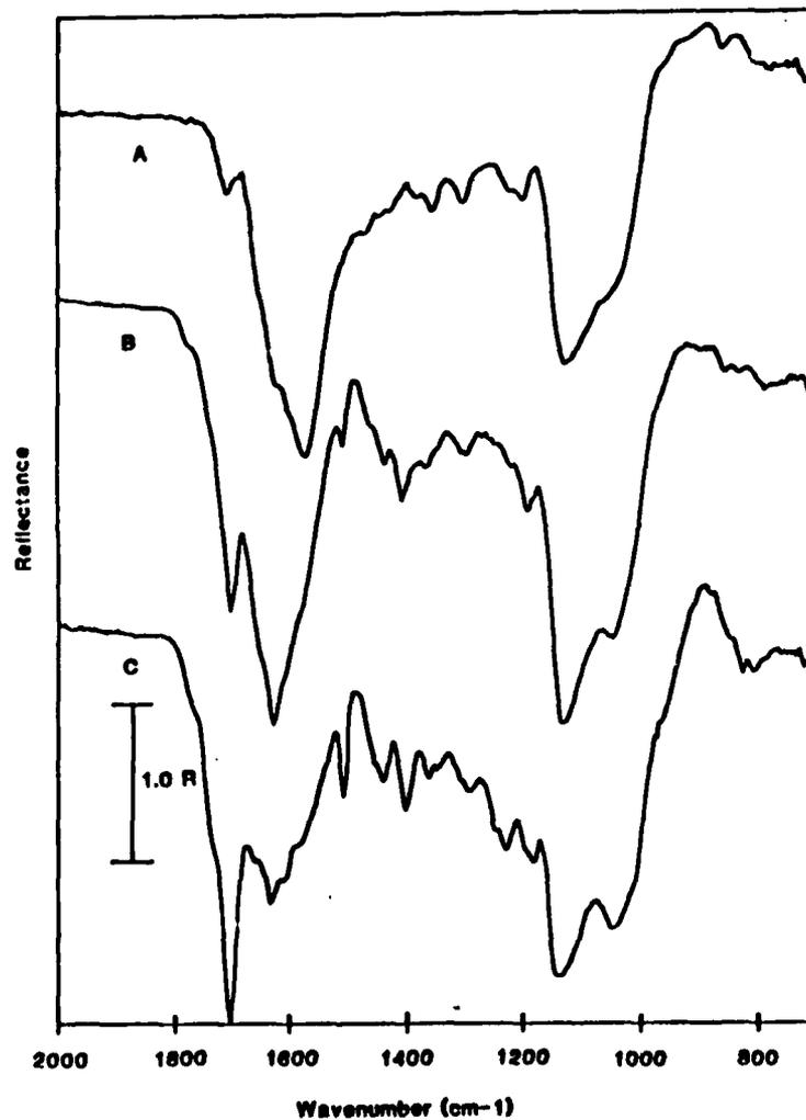
Figure 5. RAIR spectra obtained from 2024 aluminum mirrors that were primed with dilute aqueous solutions of  $\gamma$ -APS and then reacted with a mixture of epoxy resin and nadic methyl anhydride (NMA) at (A) - 75°C for one hour, (B) - 150°C for one hour, and (C) - 150°C for three hours and then rinsed with methylethylketone.
