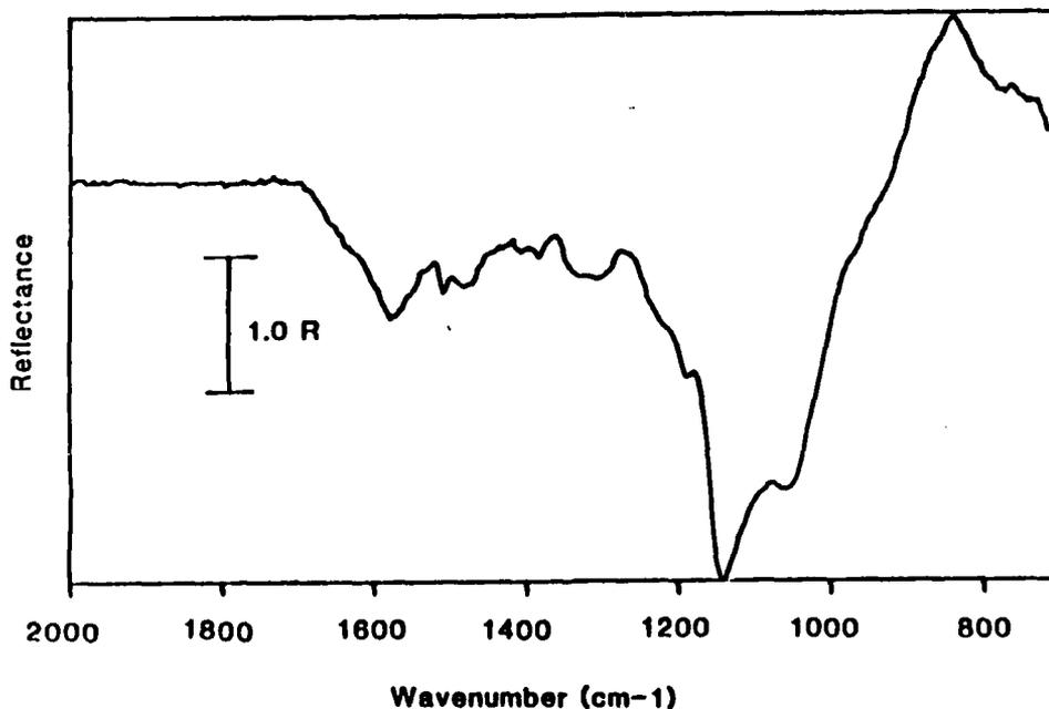
Figure 2. RAIR infrared spectrum of the substrate failure surface of a DCB specimen prepared from a steel substrate and an epoxy cured at  $75^{\circ}\text{C}$  for one hour with a tertiary amine. The substrate was primed with a dilute aqueous solution of  $\gamma$ -APS.
