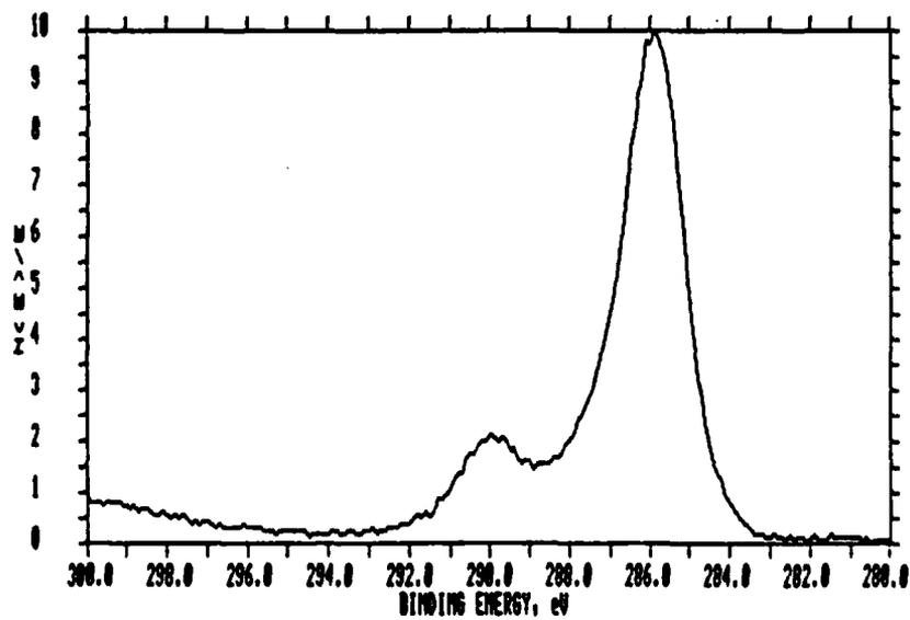
Figure 11. C(1s) XPS multiplex spectrum obtained from an NMA film coated on a 2024 aluminum mirror, heated at 150°C for two hours, and rinsed with acetone.
