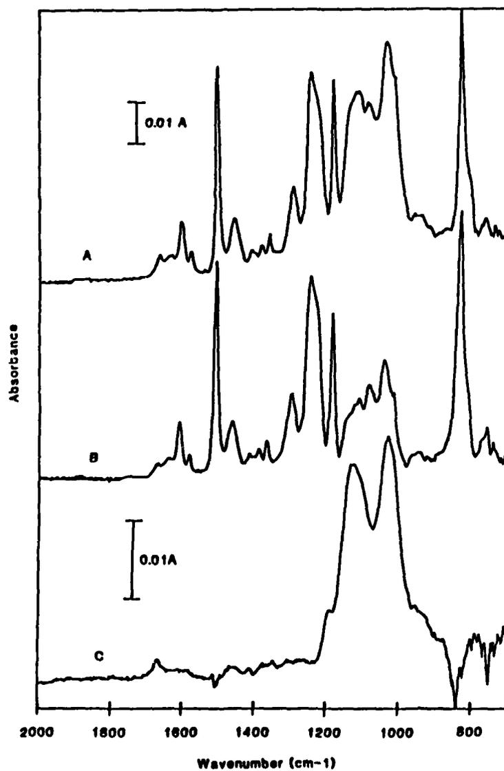
Figure 4. ATR infrared spectra of the adhesive failure surfaces of DCB specimens prepared from steel substrates and the epoxy cured with a tertiary amine at 150°C for one hour; (A) - substrate primed with a dilute aqueous solution of  $\gamma$ -APS, (B) - substrate unprimed, and (C) - the difference of A and B.
