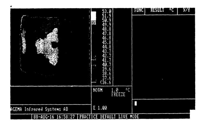
Fig. 3 This picture shows the thermal image of a concrete specimen tested under compression. The different colors indicate different temperatures. The light shaded areas represent the areas where cracking occurred first.
