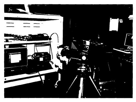
Fig. 1 Thermovision System Used to Spot Cracking in Concrete Cylinders Subjected to Compressive Loading
