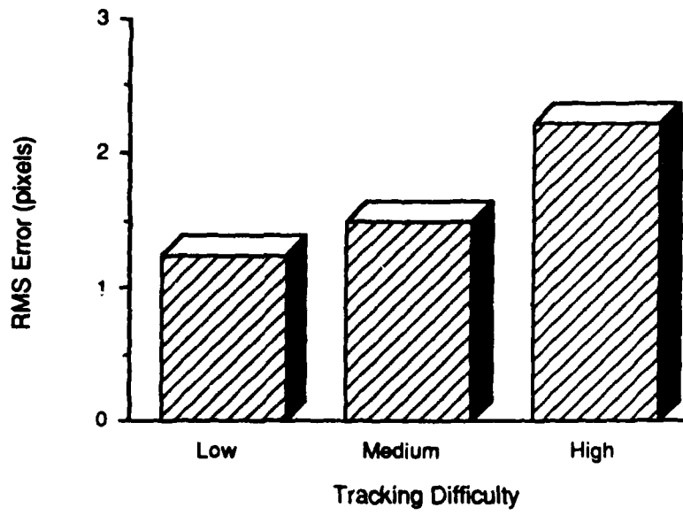
Figure 26. RMS Tracking Error as a Function of Tracking Difficulty.
