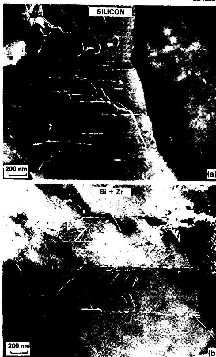
Fig. 18 Dark field TEM using [00022] reflection vector to image c+a dislocations: (a) Alloy 9, no Zr; (b) Alloy 19, high Zr.
