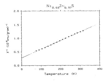
Fig. 1. Variation of magnetic susceptibility with temperature for a typical crystal of  $Ni_X Zn_{1-X}S$ . The composition  $Ni_{0.03}Zn_{0.97}S$  was calculated from the slope of the fitted line assuming the spin-only moment of 2.83 BM per Ni(II).
