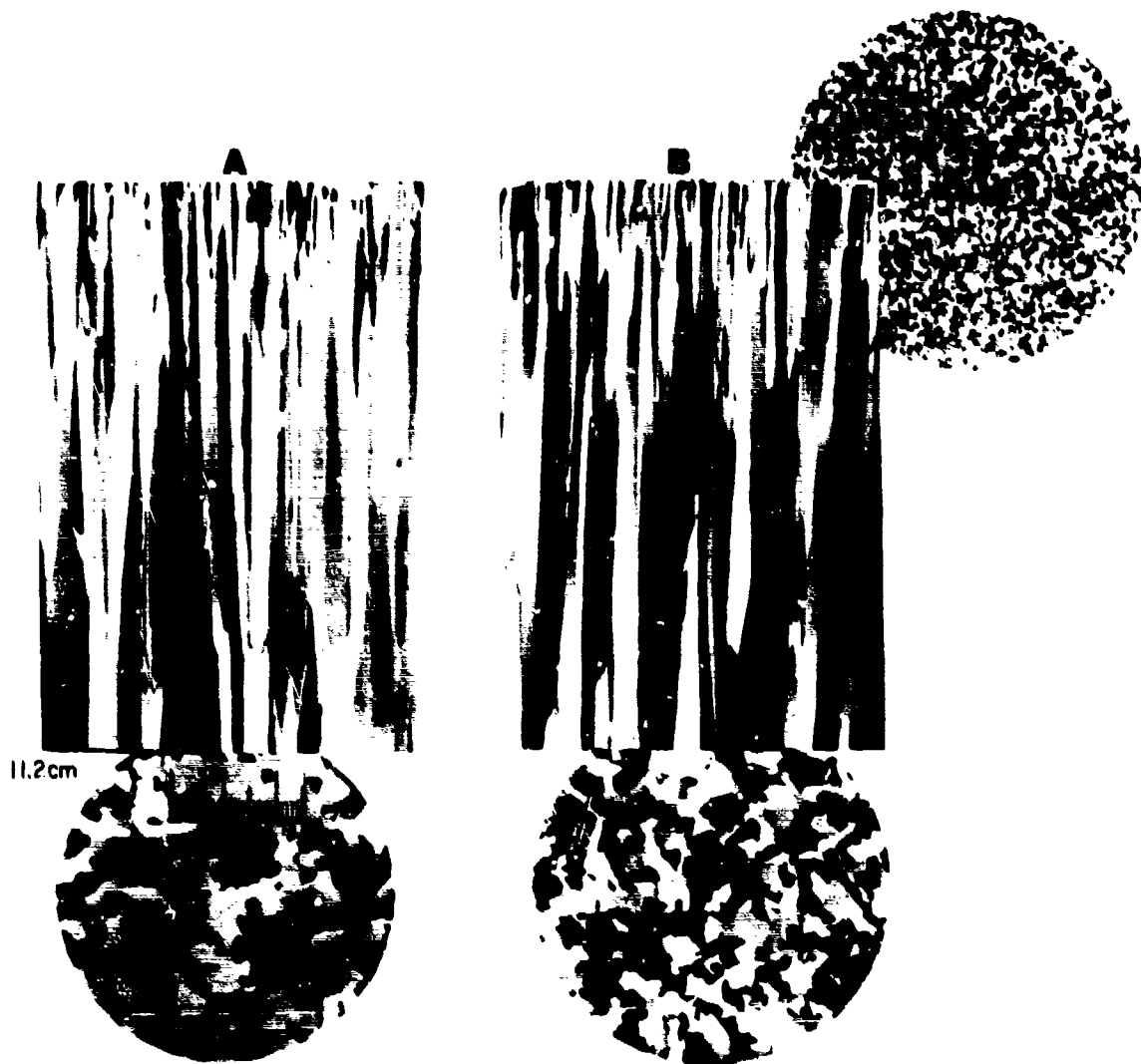
Figure 4. Vertical and horizontal thin sections of seeded (S2) columnar ice from two different locations on ice sheet 2. The crystal structures of both are essentially identical.
