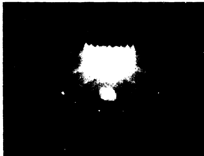
Figure 7. RHEED pattern of surface following deposition of 100 nm of undoped \text{Si}_{0.15}\text{Ge}_{0.85} on surface of Figure 5.
