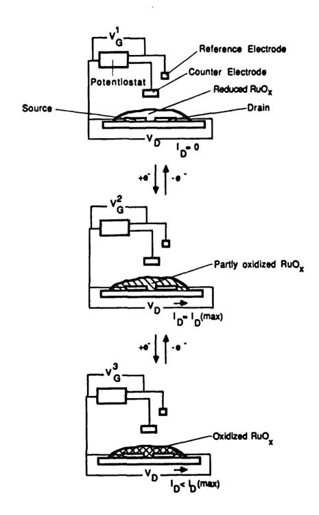
$\underline{\text{Scheme I.}} \quad \text{RuO}_{\textbf{X}}\text{-based microelectrochemical transistor.}$
