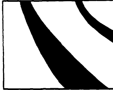
Figure 13: Interferometric measurement of wedge in \text{Bi}_{12}\text{SiO}_{20} crystal.
