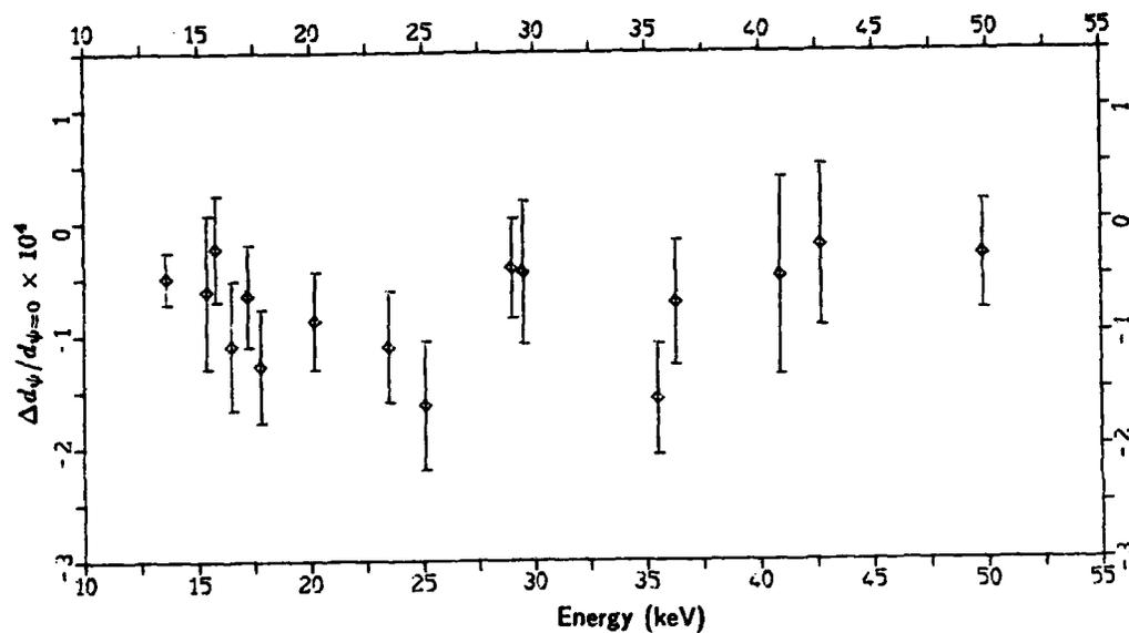
Figure 4 - Values of  $\Delta d_\psi / d_{\psi=0}$  obtained from all the reflections in the spectrum collected at  $\psi = -5.5^\circ$ . The mean value of  $\Delta d_\psi / d_{\psi=0}$  is  $-0.76 \times 10^{-4}$  with a standard deviation of  $0.44 \times 10^{-4}$ .
