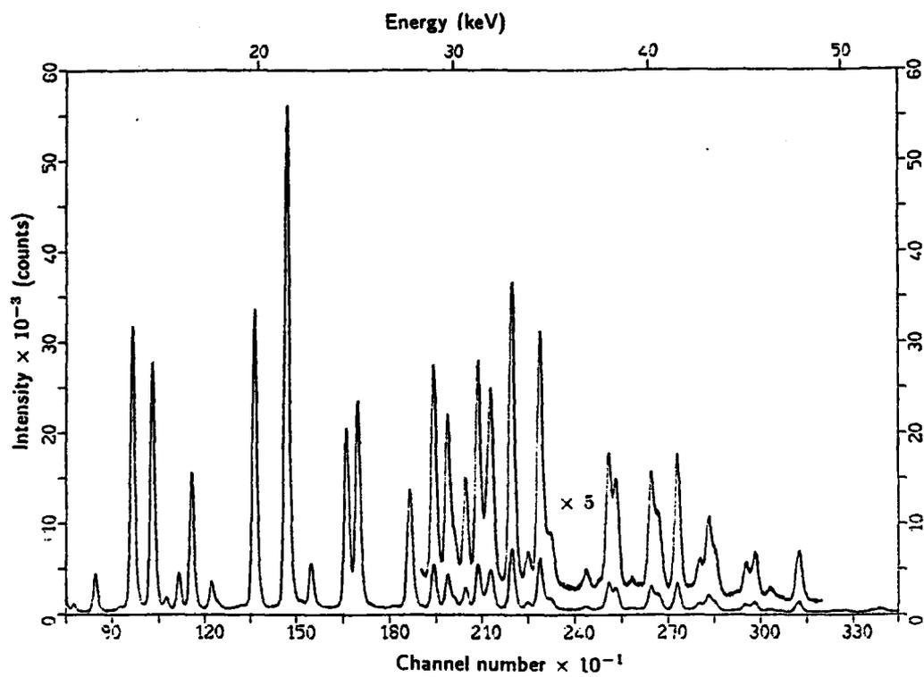
**Figure 2 - Energy dispersive spectrum of  $\text{Cr}_2\text{O}_3$  used to calibrate the diffractometer. This spectrum was collected in reflection from a rotating powder sample in 45 minutes with the SRS operating at 2 GeV and a mean current of 115 mA. The angle of diffraction  $2\theta$  was calculated as  $19.8652^\circ \pm 0.0066^\circ$  using 32 reflections.**
