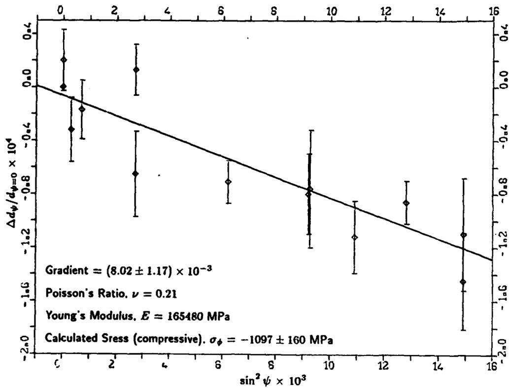
**Figure 5 - Strain versus  $\sin^2 \psi$ .** The values of  $\Delta d_{\psi} / d_{\psi=0}$  plotted are the means calculated from up to 15 reflections in a spectrum. The tilt  $\psi$  was varied from  $-7.0^\circ$  to  $+7.0^\circ$ . The straight line is the result of a least-squares fit. The values of the elastic constants for uranium were taken from reference [15].
