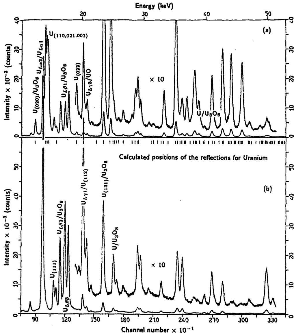
Figure 3 - Two spectra used to calculate the residual stress. The tilt angle  $\psi$  were  $-5.5^\circ$  and  $+5.5^\circ$  for (a) and (b) respectively. Both spectra were collected in 30 minutes at 2 GeV and a beam current of approximately 100 mA. The calculated positions of the reflections for uranium at  $2\theta = 19.8652^\circ$  are shown for comparison.
