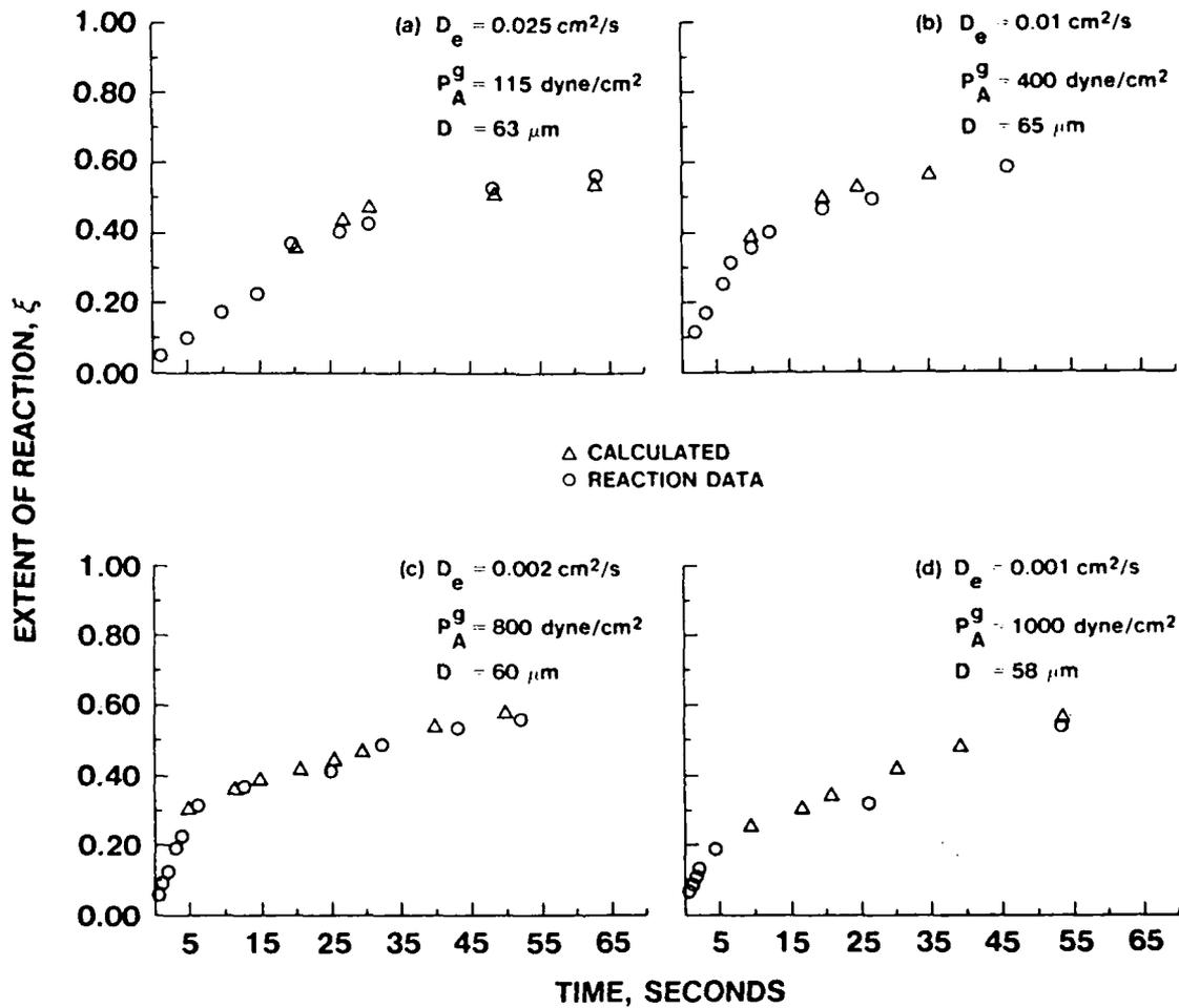
Figure 4. Comparison of Measured Extent of Reaction (O) and Theoretical Porous Shell Diffusion-Controlled Extent of Reaction (Δ) for Different Reaction Conditions. Porous Shell Diffusion-Controlled Reactions Initiated at Particle Crystallization.
