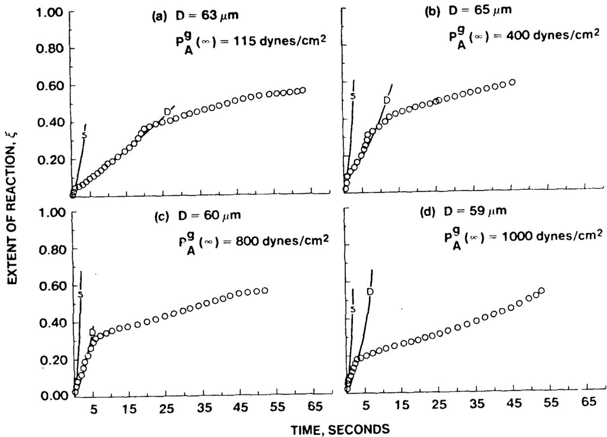
Figure 1. Comparison of Measured Extent of Reaction ( $\xi$ ) and Theoretical Surface Phase (S) and Gas Phase Diffusion-Controlled (D) Extent of Reaction for Phosphoric Acid Droplets Immersed in Ammonia Gas.
