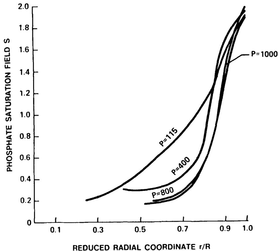
Figure 2. Theoretical Ammonium Phosphate Saturation Field Inside a Phosphoric Acid Droplet Reacting with Ammonia Gas (Ammonia gas pressure  $P$  is in units of  $\text{dyn/cm}^2$ ).
