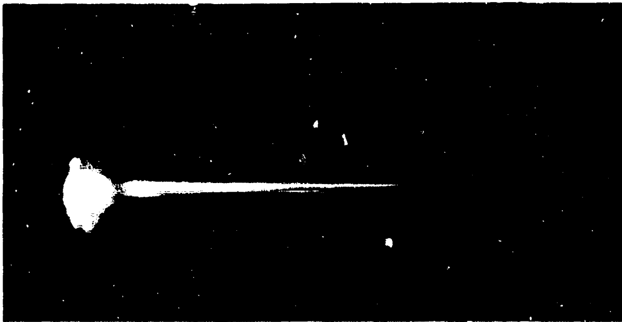
Figure 21. Ball, Tracer Flash Geometry, Long Burst
