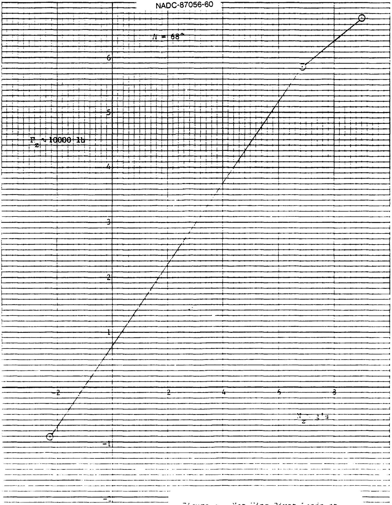
Figure 6. Net Wing Pivot Loads at 68^\circ Sweep
