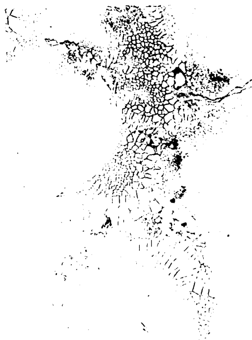
Figure 3.28: Photomicrographs selected to show appearance of eutectic constituent in unmodified Mar-M200 + 2% Hf (50% lactic acid, 33% HCL, 17% HNO 3 , 500X). Top left: G-25B, high G, low R, high G/R. Top right: G-25T, high G, high R, high \epsilon . Bottom left: G-28B, low G, low R, low \epsilon . Bottom right: G-28T, low G, high R, low G/R.
