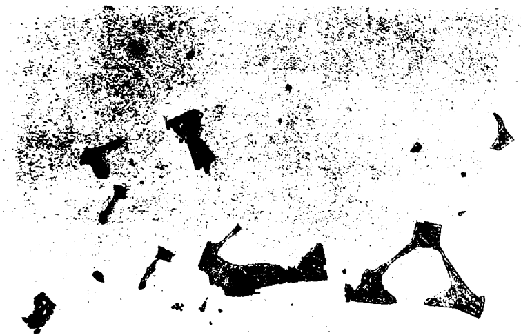
Figure 6.3a: Longitudinal view of platform region. Unetched. Vendor A, first turbine blade, 500X.
