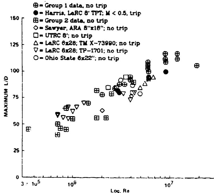
Fig. 11. Maximum lift-to-drag ratio vs. Reynolds number;  $M < 0.5$ .
