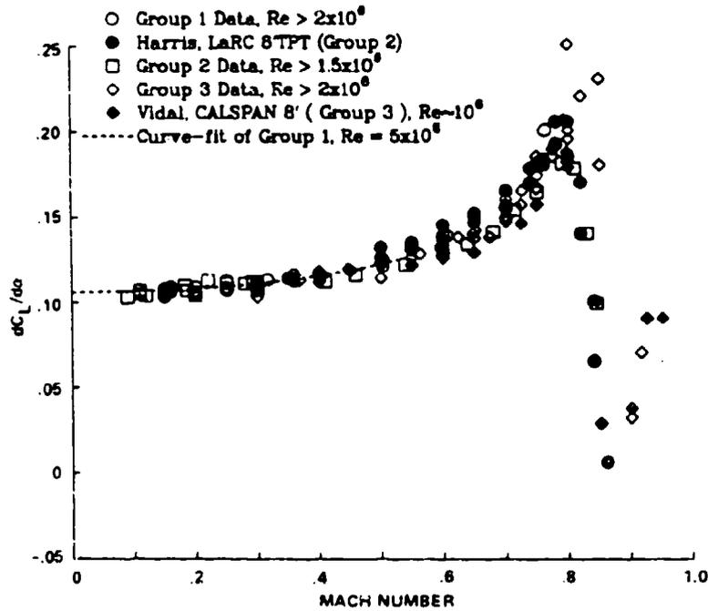
Fig. 6. Lift-curve slope vs. Mach number.
