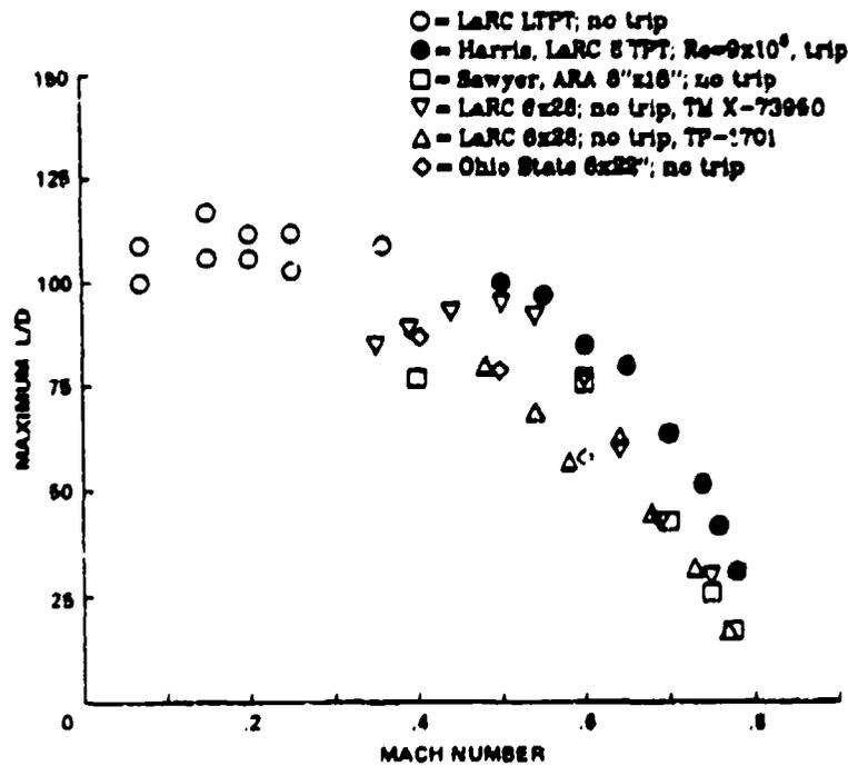
Fig. 12. Maximum lift-to-drag ratio vs. Mach number;  $4 \cdot 10^6 < Re < 9 \cdot 10^6$ .
