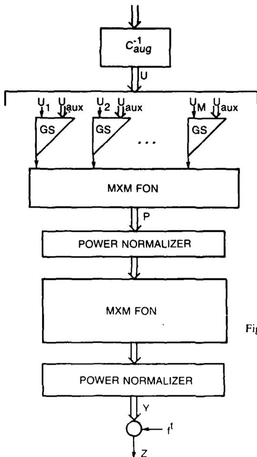
Fig. 15 - Functional equivalent of canceller seen in Fig. 11
