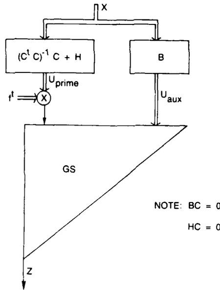
Fig. 18 — Special case of the linearly constrained canceller implementation
