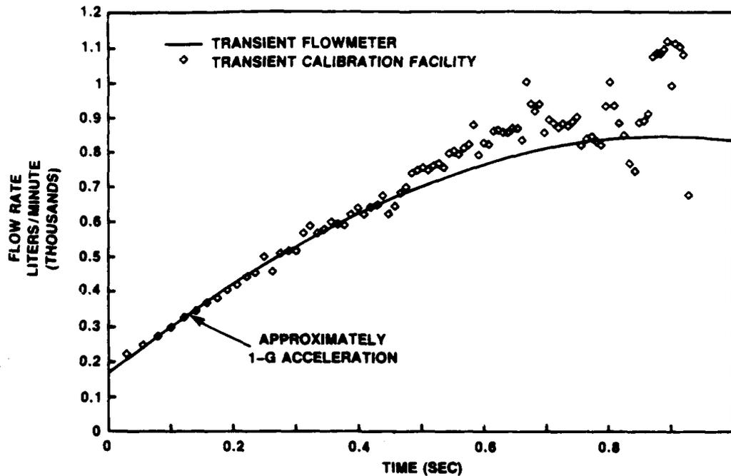
Figure II-4. Transient Flowmeter Typical Transient Calibration Curve
