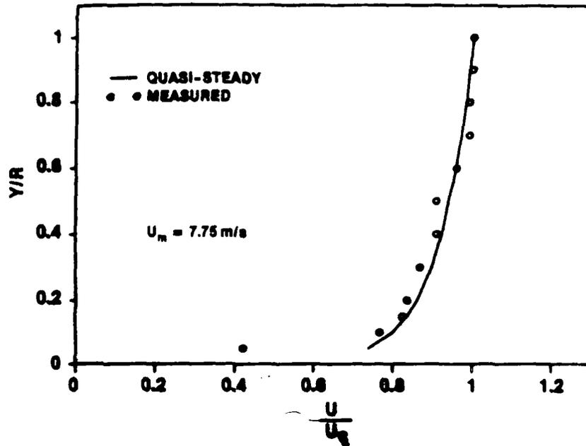
Figure IV-60i. Velocity Profile at  $t = 1.900$  s ( $t^* = 0.00176$ ) for  $\ddot{X} = 6.1$  m/s<sup>2</sup> and  $\bar{U}_{m0} = 0$
