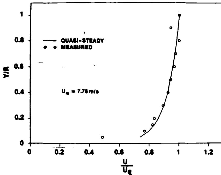
Figure 67j. Velocity Profile at  $t = 3.500$  s for  $\ddot{X} = 2.4$  m/s<sup>2</sup> and  $\bar{U}_{m0} = 1$  m/s
