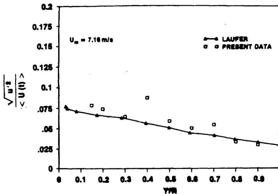
Figure IV-74b. Turbulence Intensity Profile at  $t = 1.600$  s for  $\ddot{X} = 6.1$  m/s<sup>2</sup> and  $\bar{U}_{m0} = 1$  m/s
