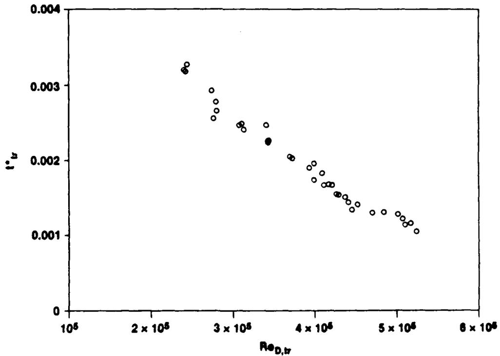
Figure IV-30. Nondimensional Time vs Pipe Reynolds Number at Transition
