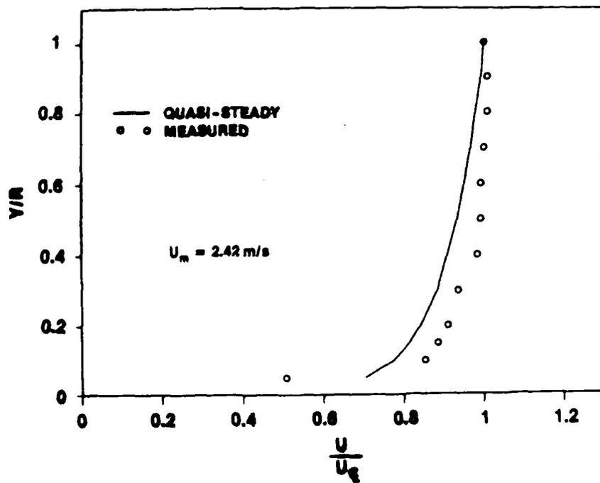
Figure IV-72b. Velocity Profile at  $t = 0.800$  s for  $\ddot{X} = 6.1$  m/s<sup>2</sup> and  $\bar{U}_{m0} = 1$  m/s
