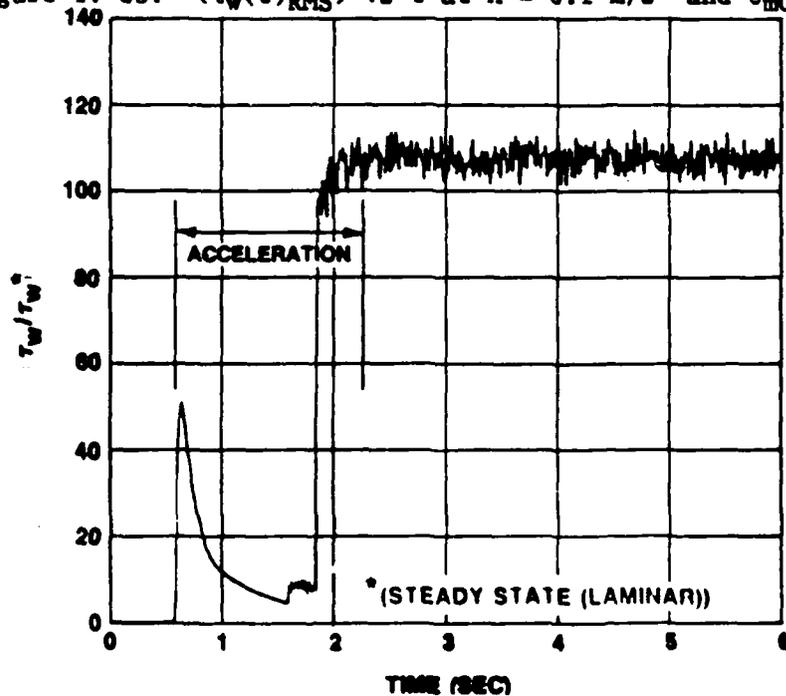
Figure IV-84.  $\tau_w$  Nondimensionalized by Quasi-Steady Laminar Value at  $\ddot{X} = 6.1 \text{ m/s}^2$  and  $\bar{U}_{m0} = 0$
