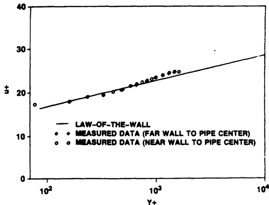
Figure IV-1. Steady-State Velocity Profile at  $Re_D = 65,000$
