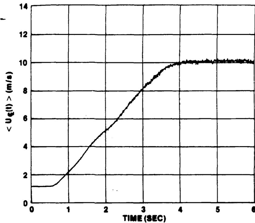
Figure IV-65.  $\langle U_{c1}(t) \rangle$  vs  $t$  for Ensemble Average of 20 Runs at  $\ddot{X} = 2.4 \text{ m/s}^2$  and  $\bar{U}_{m0} = 1 \text{ m/s}$
