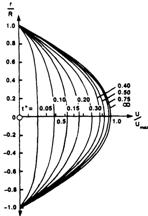
Figure I-1. Time-Dependent Velocity Profiles from Szymanski's Solution
