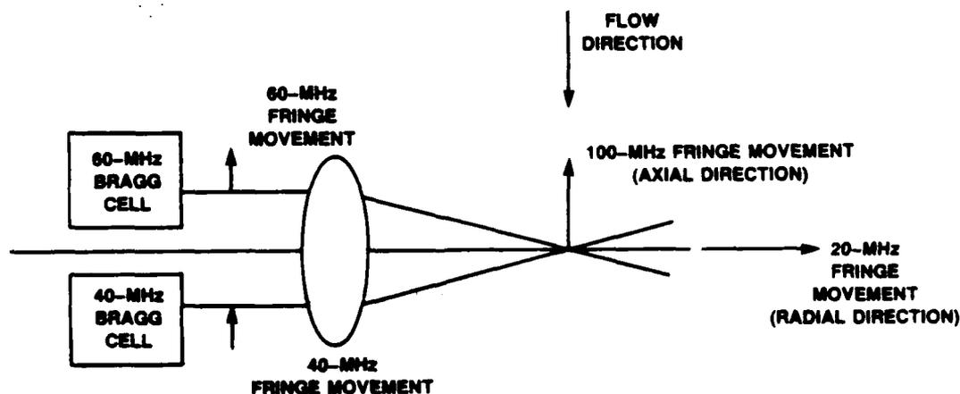
Figure II-10. Laser Doppler Velocimeter Frequency Shifting
