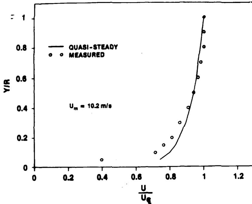
Figure IV-72g. Velocity Profile at  $t = 2.500$  s for  $\ddot{X} = 6.1$  m/s<sup>2</sup> and  $\bar{U}_{m0} = 1$  m/s
