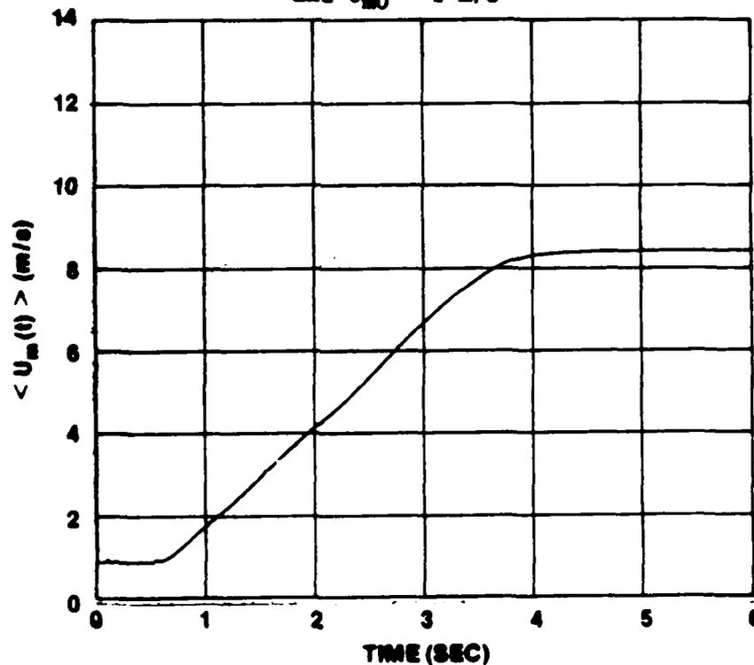
Figure IV-62.  $\langle U_m(t) \rangle$  vs  $t$  for Ensemble Average of 20 Runs at  $\ddot{X} = 2.4 \text{ m/s}^2$  and  $\bar{U}_{m0} = 1 \text{ m/s}$
