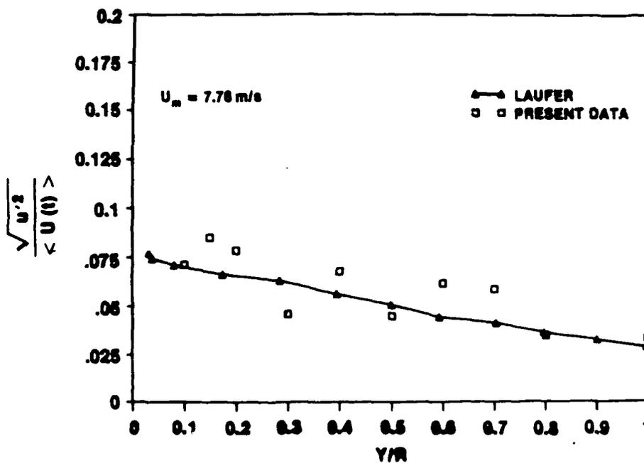
Figure IV-73f. Turbulence Intensity Profile at  $t = 3.500$  s for  $\ddot{X} = 2.4$  m/s<sup>2</sup> and  $\bar{U}_{m0} = 1$  m/s
