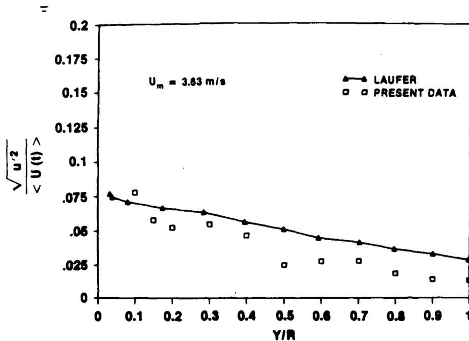
Figure IV-74a. Turbulence Intensity Profile at  $t = 1.000$  s for  $\ddot{X} = 6.1$  m/s<sup>2</sup> and  $\bar{U}_{m0} = 1$  m/s
