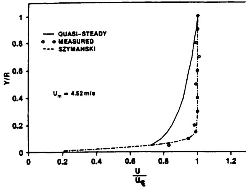
Figure IV-55e. Velocity Profile at  $t = 2.500 \text{ s}$  ( $t^* = 0.00255$ )
