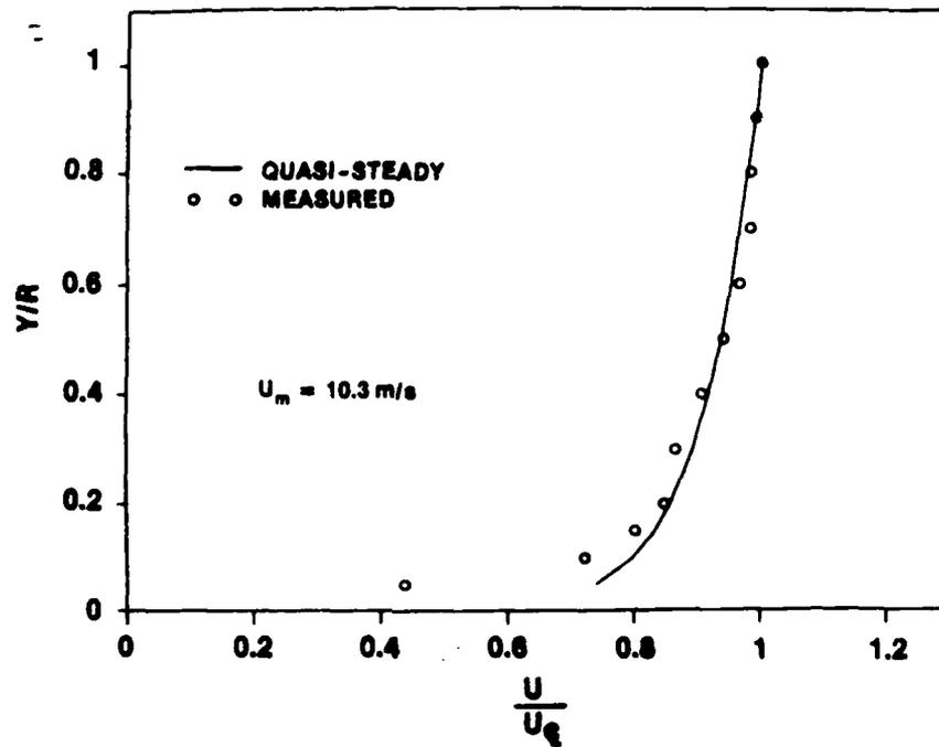
Figure IV-72i. Velocity Profile at  $t = 4.000$  s for  $\ddot{X} = 6.1$  m/s<sup>2</sup> and  $\bar{U}_{m0} = 1$  m/s
