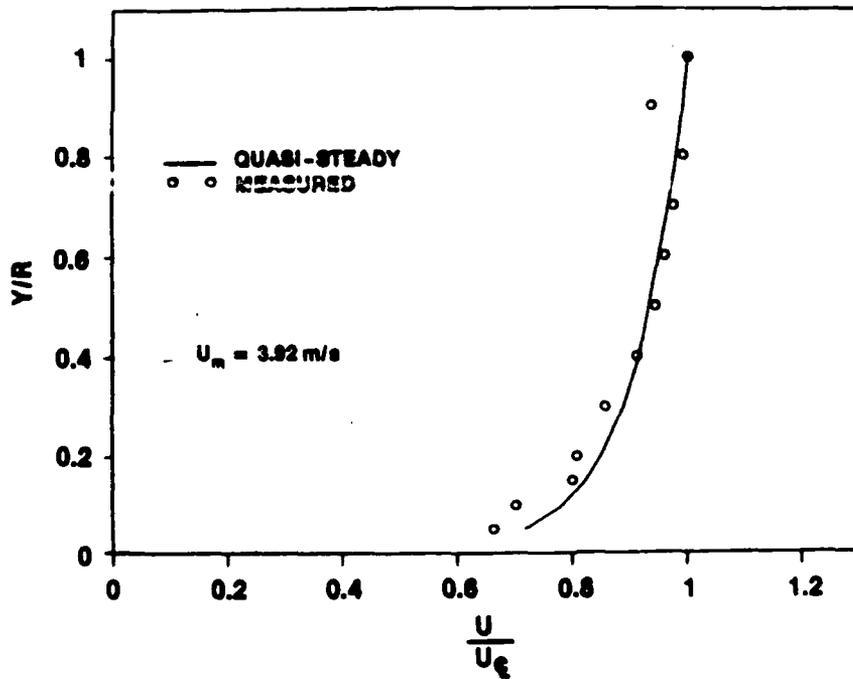
Figure 67f. Velocity Profile at  $t = 1.900$  s for  $\ddot{X} = 2.4$  m/s<sup>2</sup> and  $\bar{U}_{m0} = 1$  m/s
