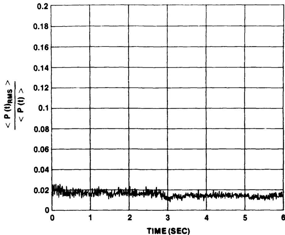
Figure IV-97.  $\langle P(t)_{RMS} \rangle$  vs  $t$  for Ensemble Average of 20 Runs at  $X = 2.4 \text{ m/s}^2$  and  $\bar{U}_{m0} = 0$
