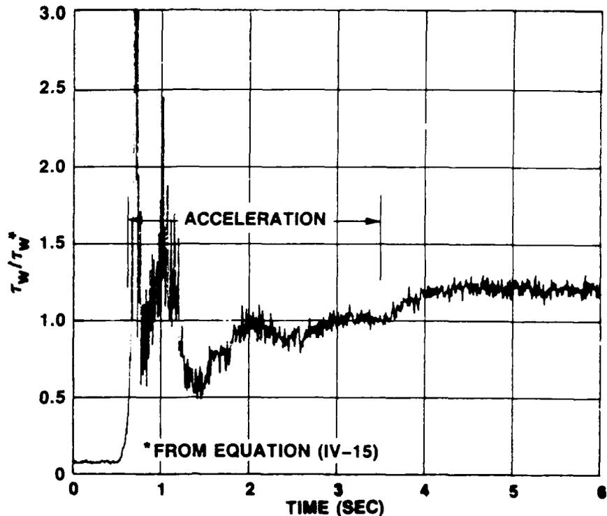
Figure IV-103.  $\tau_w$  Nondimensionalized by Equation (IV-15) for  $\dot{X} = 2.4 \text{ m/s}^2$  and  $\bar{U}_{m0} = 1 \text{ m/s}$
