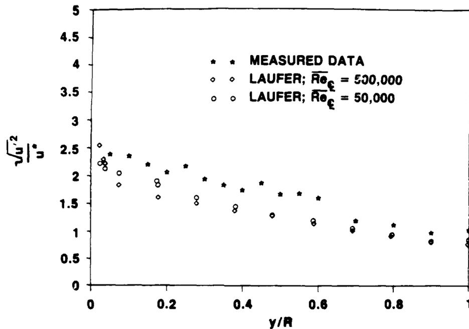
Figure IV-7. Steady-State Turbulence Intensity at  $\overline{Re}_D = 450,000$
