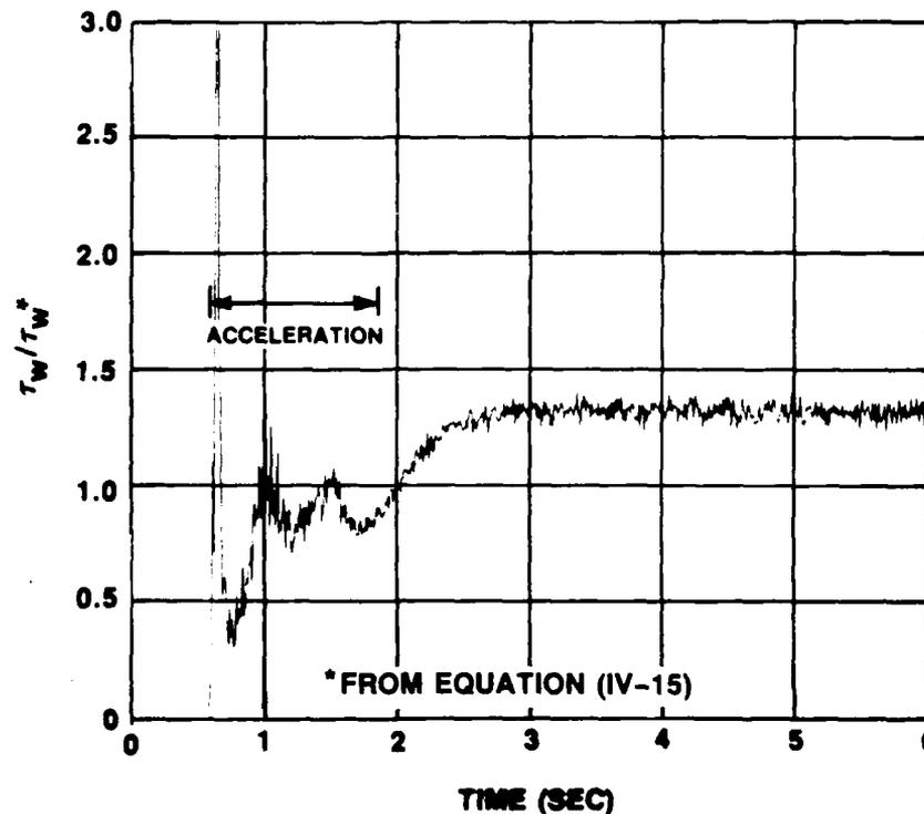
Figure IV-104.  $\tau_w$  Nondimensionalized by Equation (IV-15) for  $X = 6.1 \text{ m/s}^2$  and  $\bar{U}_{m0} = 1 \text{ m/s}$
