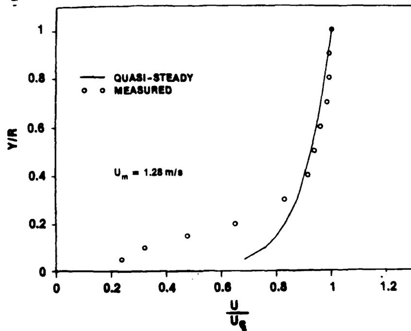
Figure IV-72a. Velocity Profile at  $t = 0.600$  s for  $\ddot{X} = 6.1$  m/s<sup>2</sup> and  $\bar{U}_{m0} = 1$  m/s
