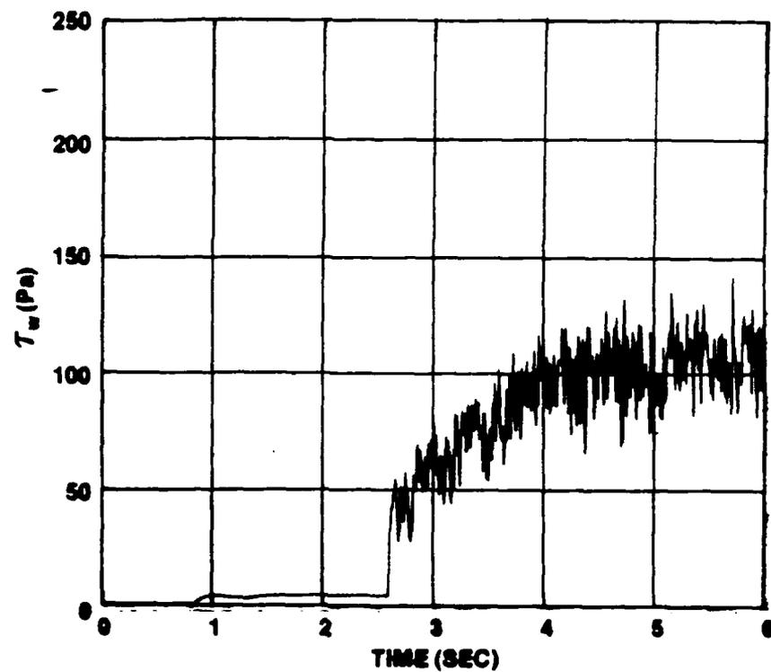
Figure IV-75.  $\tau_w$  vs  $t$  for One Typical Run at  $\ddot{X} = 2.4 \text{ m/s}^2$  and  $\bar{U}_{m0} = 0$
