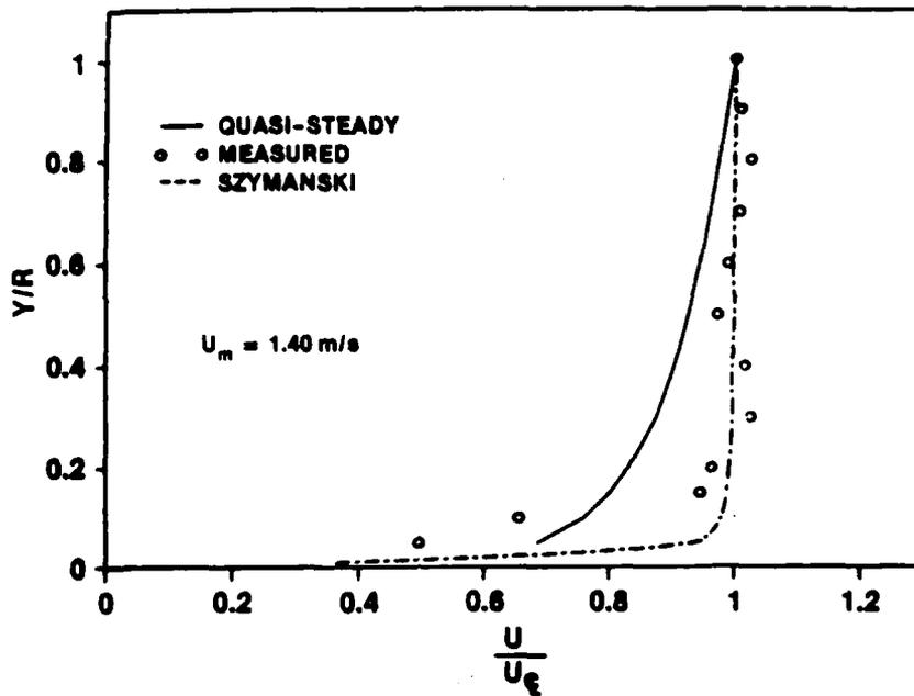
Figure IV-55a. Velocity Profile at  $t = 1.100$  s ( $t^* = 0.000792$ )
