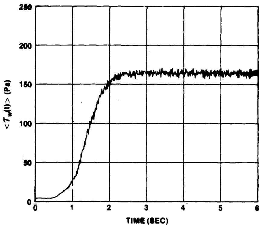
Figure IV-92.  $\langle \tau_w(t) \rangle$  vs  $t$  for Ensemble Average of 20 Runs at  $\bar{X} = 2.4 \text{ m/s}^2$  and  $\bar{U}_{m0} = 1 \text{ m/s}^2$
