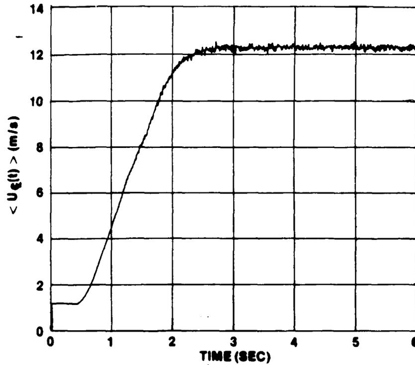
Figure IV-70.  $\langle U_{c1}(t) \rangle$  vs  $t$  for Ensemble Average of 20 Runs at  $\bar{X} = 6.1 \text{ m/s}^2$  and  $\bar{U}_{m0} = 1 \text{ m/s}$
