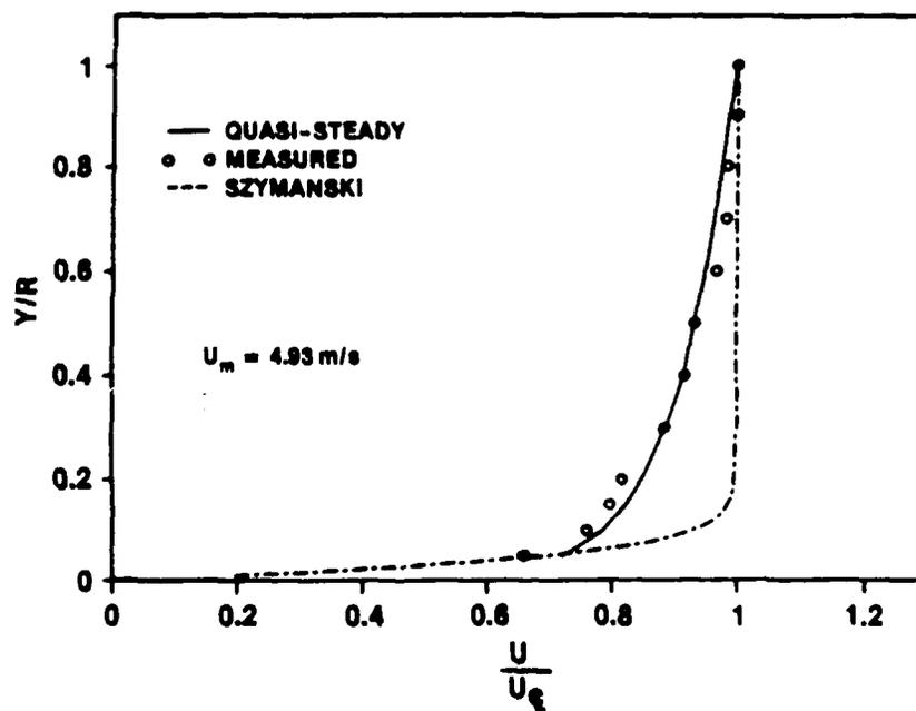
Figure 55l. Velocity Profile at  $t = 2.700$  s ( $t^* = 0.00278$ )
