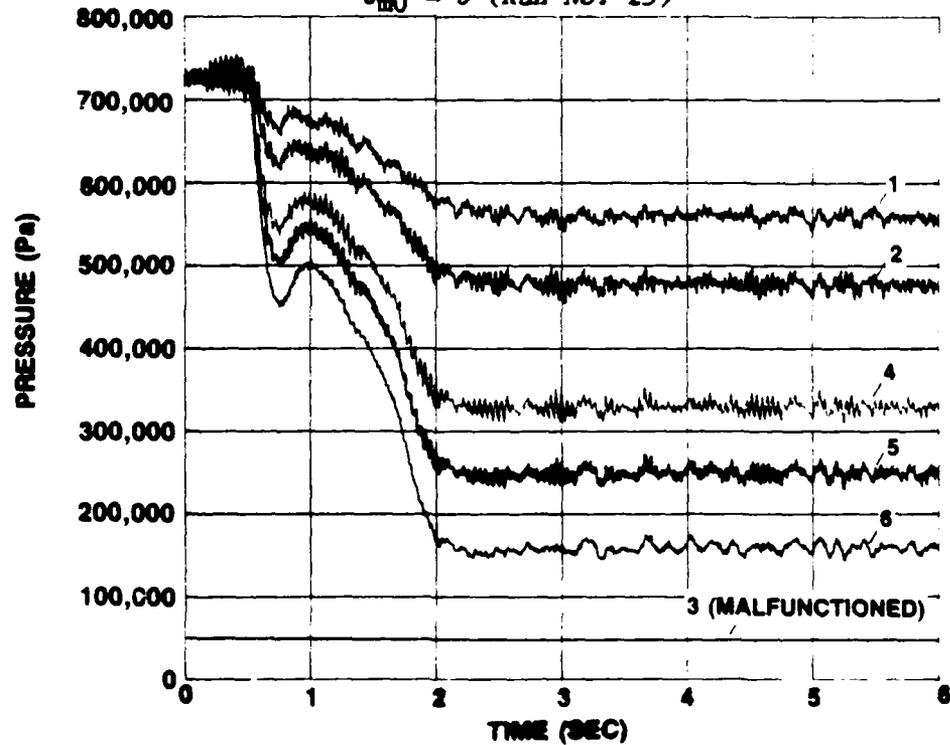
Figure IV-24. Pressure vs  $t$  for  $\ddot{X} = 6.53 \text{ m/s}^2$  and  $\bar{U}_{m0} = 0$  (Run No. 25)
