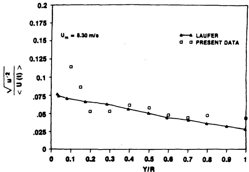
Figure 73g. Turbulence Intensity Profile at  $t = 4.000$  s for  $\dot{X} = 2.4$  m/s<sup>2</sup> and  $\bar{U}_{m0} = 1$  m/s
