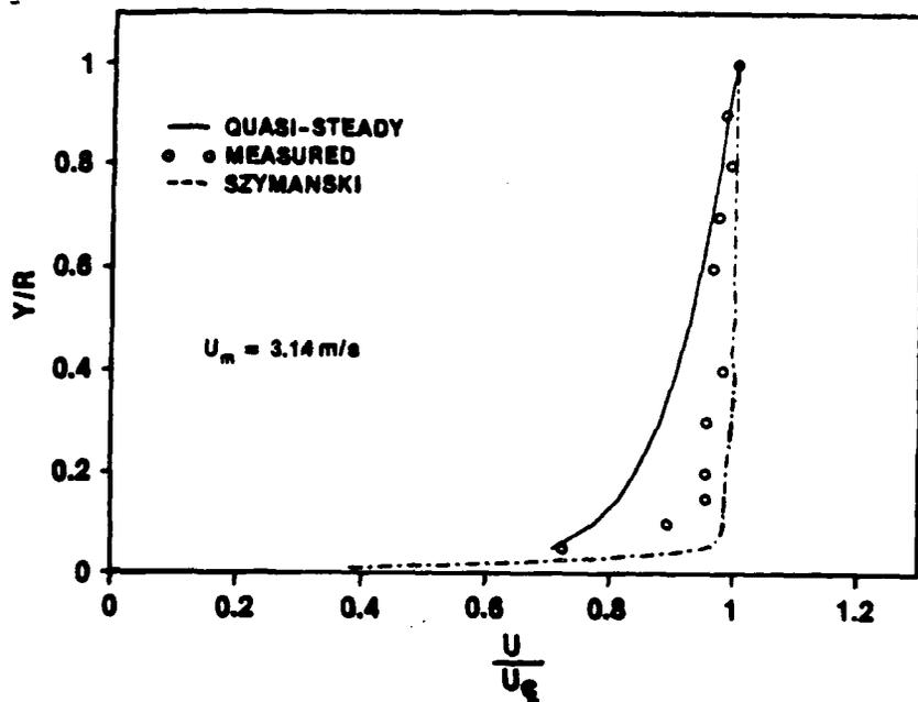
Figure IV-60a. Velocity Profile at  $t = 1.100$  s ( $t^* = 0.000713$ )
