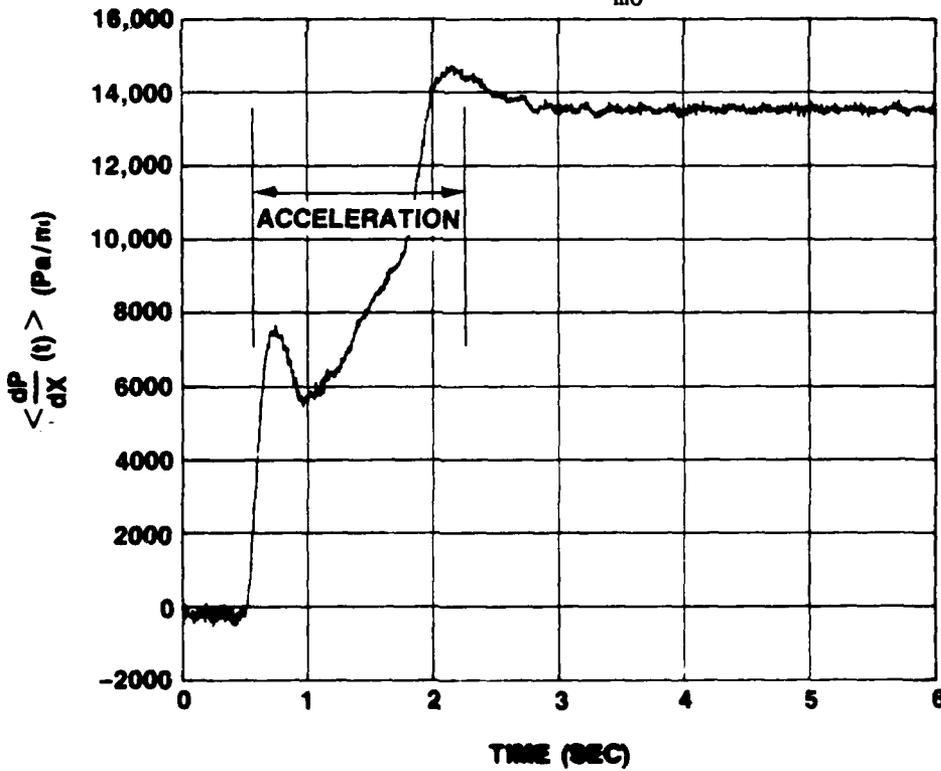
Figure IV-99.  $\langle dp/dx(t) \rangle$  vs  $t$  for Ensemble Average of 20 runs at  $\dot{X} = 6.1 \text{ m/s}^2$  and  $\bar{U}_{m0} = 0$
