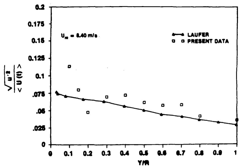
Figure IV-73h. Turbulence Intensity Profile at  $t = 5.000$  s for  $\dot{X} = 2.4$  m/s<sup>2</sup> and  $\bar{U}_{m0} = 1$  m/s
