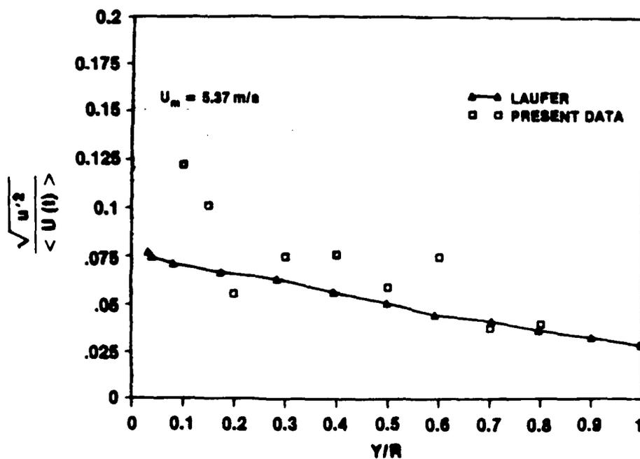
Figure IV-73d. Turbulence Intensity Profile at  $t = 2.500$  s for  $\bar{X} = 2.4$  m/s<sup>2</sup> and  $\bar{U}_{m0} = 1$  m/s
