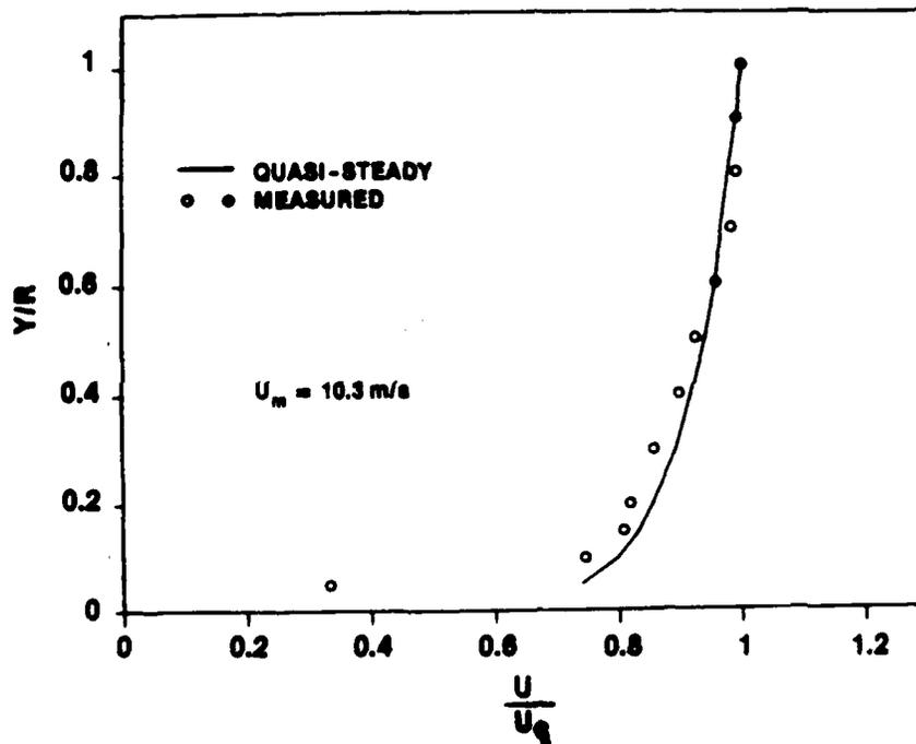
Figure IV-72h. Velocity Profile at  $t = 3.000$  s for  $\ddot{X} = 6.1$  m/s<sup>2</sup> and  $\bar{U}_{m0} = 1$  m/s
