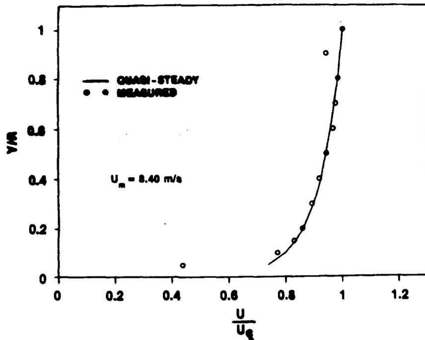
Figure 67l. Velocity Profile at  $t = 5.000$  s for  $\ddot{X} = 2.4$  m/s<sup>2</sup> and  $\bar{U}_{m0} = 1$  m/s
