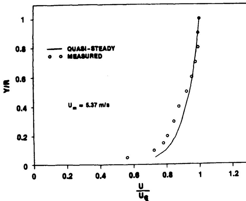
Figure IV-72d. Velocity Profile at  $t = 1.300$  s for  $\ddot{X} = 6.1$  m/s<sup>2</sup> and  $\bar{U}_{m0} = 1$  m/s
