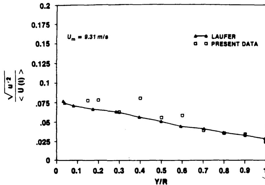
Figure IV-74c. Turbulence Intensity Profile at  $t = 2.000$  s for  $\dot{X} = 6.1$  m/s<sup>2</sup> and  $\bar{U}_{m0} = 1$  m/s
