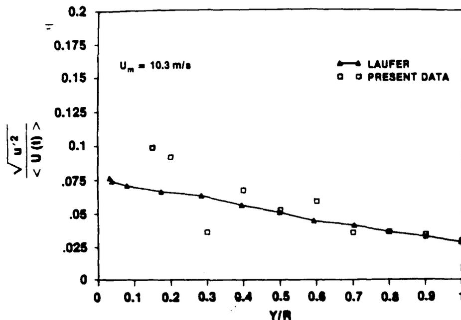
Figure IV-74e. Turbulence Intensity Profile at  $t = 5.900$  s for  $\dot{X} = 6.1$  m/s<sup>2</sup> and  $\bar{U}_{m0} = 1$  m/s
