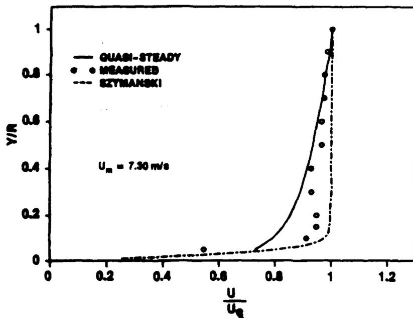
Figure IV-60f. Velocity Profile at  $t = 1.800 \text{ s}$  ( $t^* = 0.00166$ )
