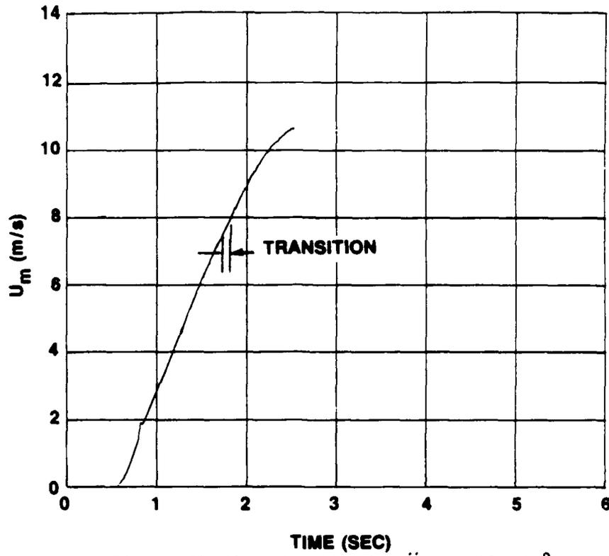
Figure IV-21.  $U_m$  vs  $t$  for  $\ddot{X} = 6.53 \text{ m/s}^2$  and  $\bar{U}_{m0} = 0$  (Run No. 25)
