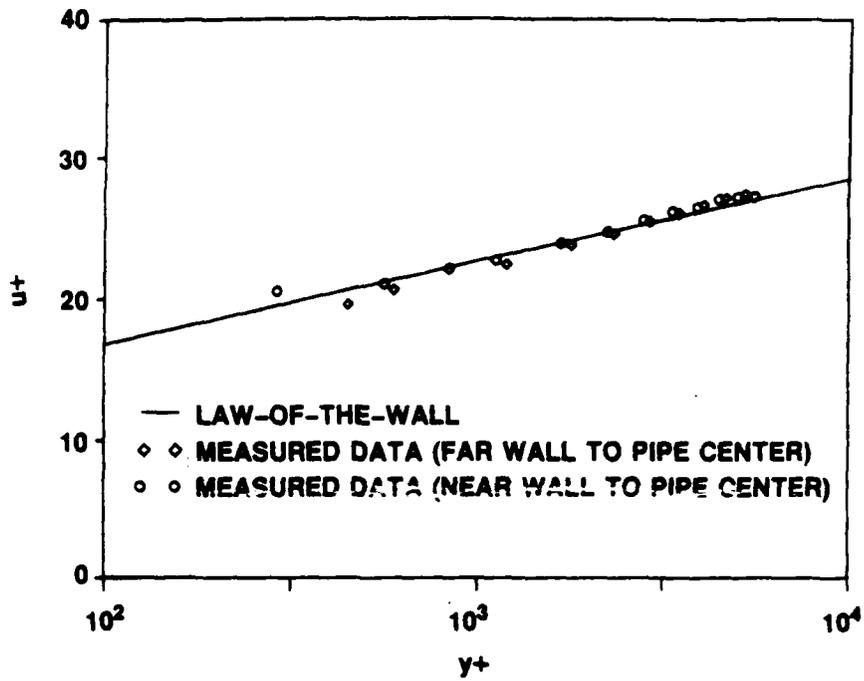
Figure IV-2. Steady-State Velocity Profile at  $Re_D = 275,000$
