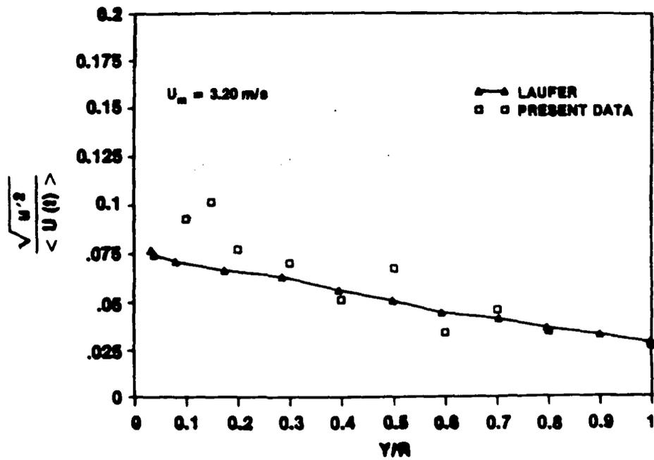
Figure IV-73b. Turbulence Intensity Profile at  $t = 1.600$  s for  $\dot{X} = 2.4$  m/s<sup>2</sup> and  $\bar{U}_{m0} = 1$  m/s
