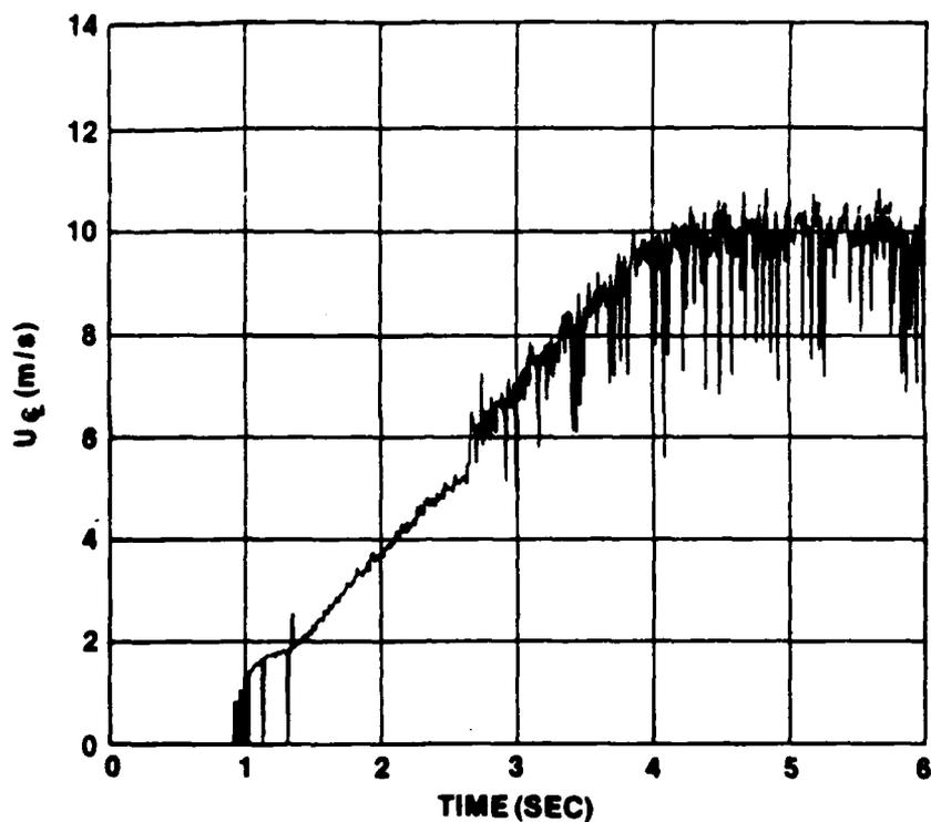
Figure IV-50.  $U_{c1}$  vs  $t$  for One Typical Run at  $\ddot{X} = 2.4 \text{ m/s}^2$  and  $\bar{U}_{m0} = 0$
