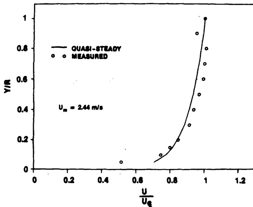
Figure 67d. Velocity Profile at  $t = 1.300$  s for  $\ddot{X} = 2.4$  m/s<sup>2</sup> and  $\bar{U}_{m0} = 1$  m/s
