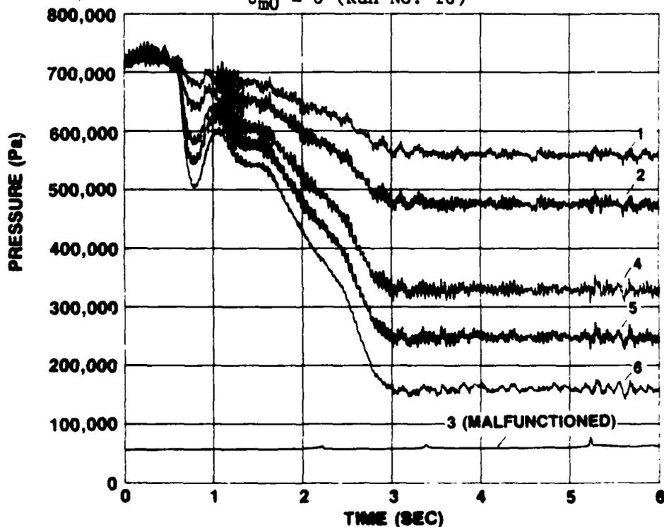
Figure IV-16. Pressure vs  $t$  for  $\ddot{X} = 4.36 \text{ m/s}^2$  and  $\bar{U}_{m0} = 0$  (Run No. 16)
