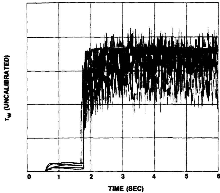
Figure IV-23.  $\tau_w$  vs  $t$  for  $\ddot{X} = 6.53 \text{ m/s}^2$  and  $\bar{U}_{m0} = 0$  (Run No. 25)
