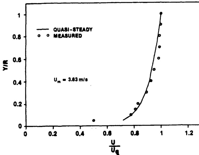
Figure IV-72c. Velocity Profile at  $t = 1.000$  s for  $\ddot{X} = 6.1$  m/s<sup>2</sup> and  $\bar{U}_{m0} = 1$  m/s
