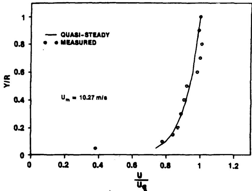
Figure IV-60k. Velocity Profile at  $t = 3.000$  s for  $\ddot{X} = 6.1$  m/s<sup>2</sup> and  $\bar{U}_{m0} = 0$
