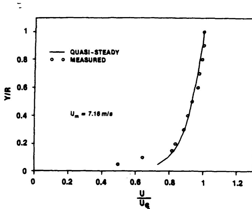
Figure IV-72e. Velocity Profile at  $t = 1.600$  s for  $\ddot{X} = 6.1$  m/s<sup>2</sup> and  $\bar{U}_{m0} = 1$  m/s
