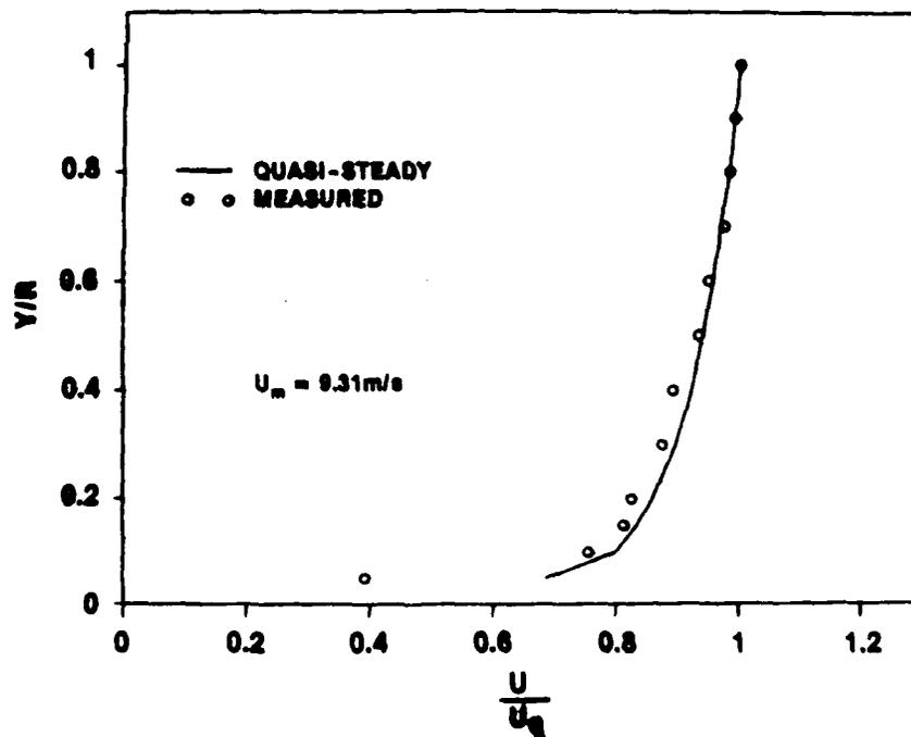
Figure IV-72f. Velocity Profile at  $t = 2.000$  s for  $\ddot{X} = 6.1$  m/s<sup>2</sup> and  $\bar{U}_{m0} = 1$  m/s
