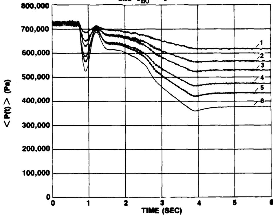
Figure IV-96.  $\langle P(t) \rangle$  vs  $t$  for Ensemble Average for 20 Runs at  $\dot{X} = 2.4 \text{ m/s}^2$  and  $\bar{U}_{m0} = 0$
