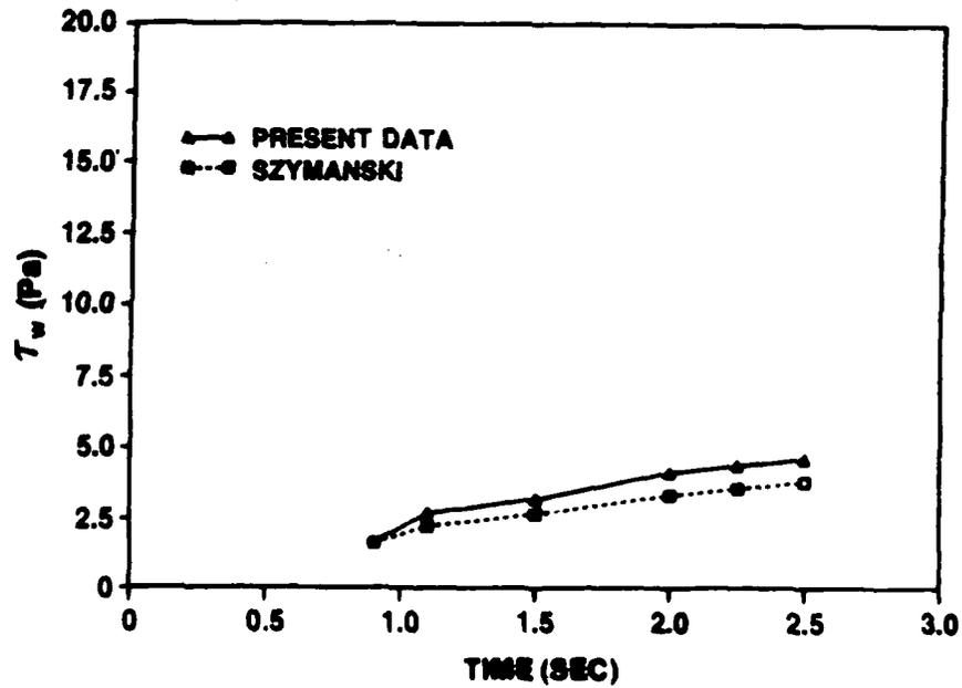
Figure IV-80. Comparison of  $\tau_w$  Measured with Szymanski's Solution at  $\ddot{X} = 2.4 \text{ m/s}^2$  and  $U_{m0} = 0$
