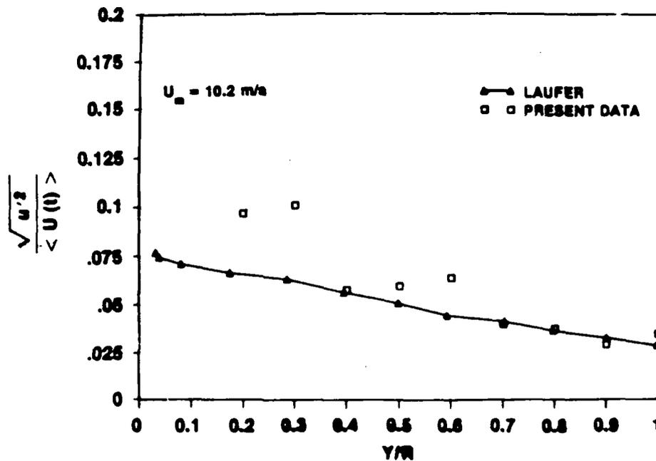
Figure IV-74d. Turbulence Intensity Profile at  $t = 2.500$  s for  $\dot{X} = 6.1$  m/s<sup>2</sup> and  $\bar{U}_{m0} = 1$  m/s
