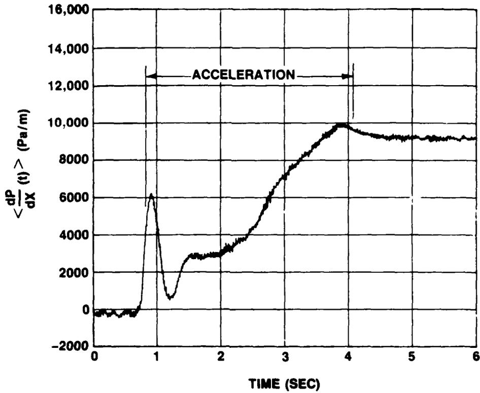
Figure IV-98.  $\langle dp/dx(t) \rangle$  vs  $t$  for Ensemble Average of 20 runs at  $\dot{X} = 2.4 \text{ m/s}^2$  and  $\bar{U}_{m0} = 0$
