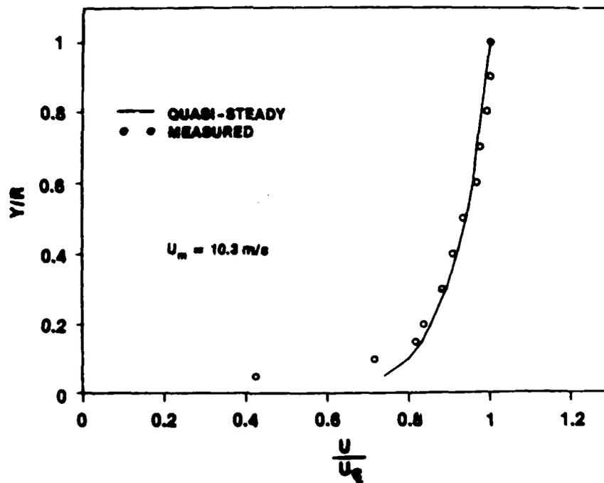
Figure IV-72j. Velocity Profile at  $t = 5.000$  s for  $\ddot{X} = 6.1$  m/s<sup>2</sup> and  $\bar{U}_{m0} = 1$  m/s
