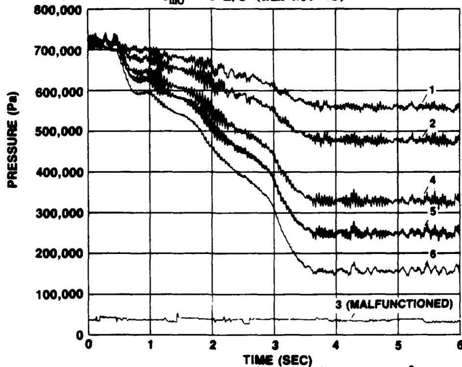
Figure IV-38. Pressure vs  $t$  for  $\ddot{X} = 3.00 \text{ m/s}^2$  and  $\bar{U}_{m0} = 1 \text{ m/s}$  (Run No. 41)
