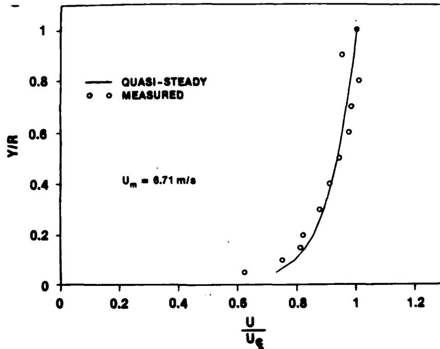
Figure 67i. Velocity Profile at  $t = 3.000$  s for  $\ddot{X} = 2.4$  m/s<sup>2</sup> and  $\bar{U}_{m0} = 1$  m/s
