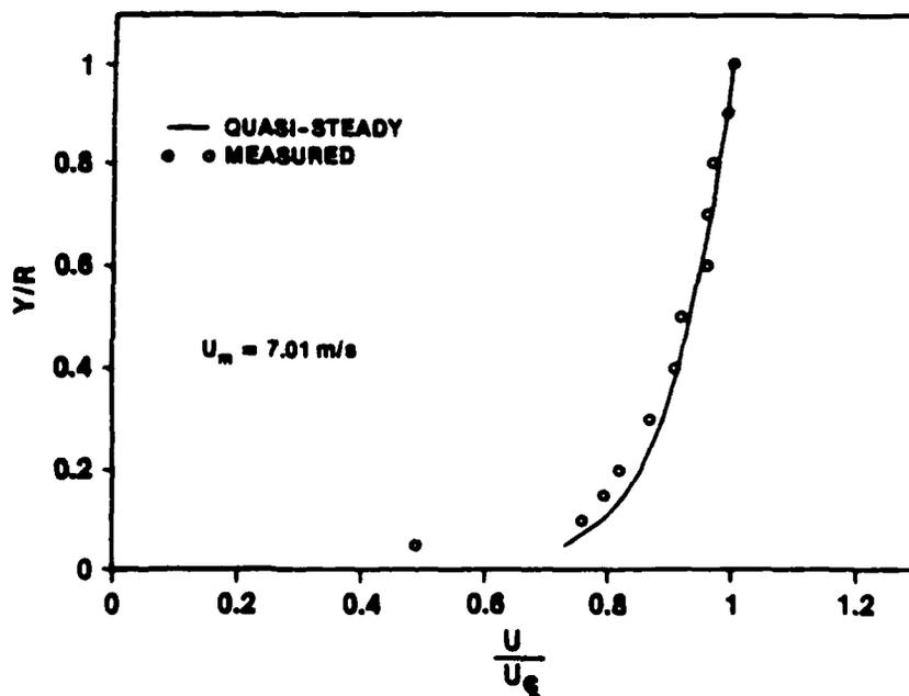
Figure 55n. Velocity Profile at  $t = 3.500$  s ( $t^* = 0.00396$ ) for  $\ddot{X} = 2.4$  m/s<sup>2</sup> and  $\bar{U}_{m0} = 0$
