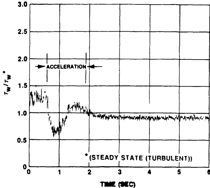
Figure IV-94.  $\tau_w$  Nondimensionalized by Quasi-Steady Turbulent Value at  $\dot{X} = 2.4 \text{ m/s}^2$  and  $\bar{U}_{m0} = 1 \text{ m/s}^2$
