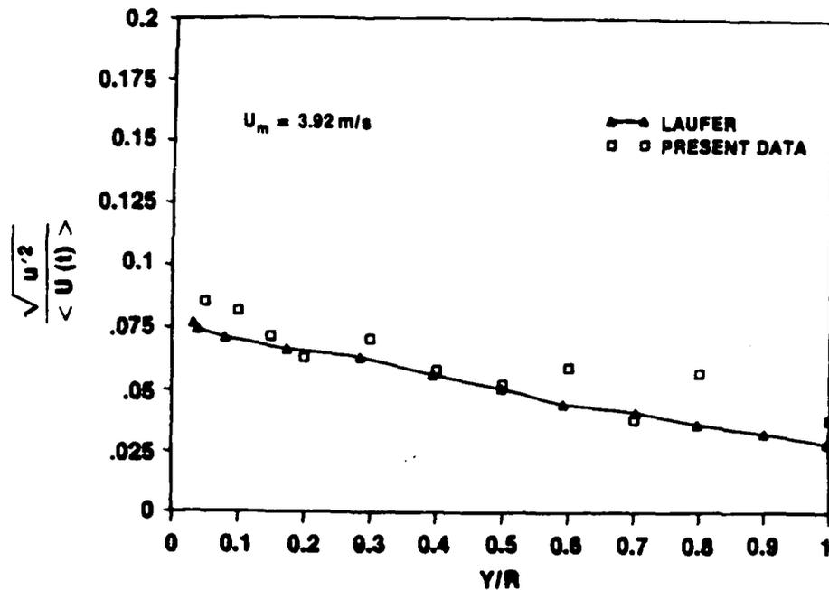
Figure IV-73c. Turbulence Intensity Profile at  $t = 1.900$  s for  $\bar{X} = 6.1$  m/s<sup>2</sup> and  $\bar{U}_{m0} = 1$  m/s
