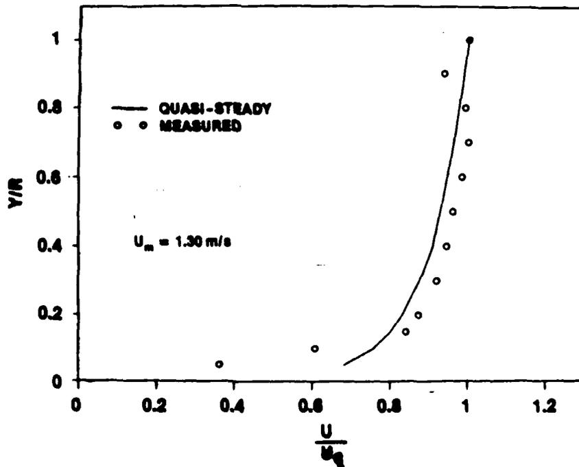
Figure 67b. Velocity Profile at  $t = 0.800$  s for  $\ddot{X} = 2.4$  m/s<sup>2</sup> and  $\bar{U}_{m0} = 1$  m/s
