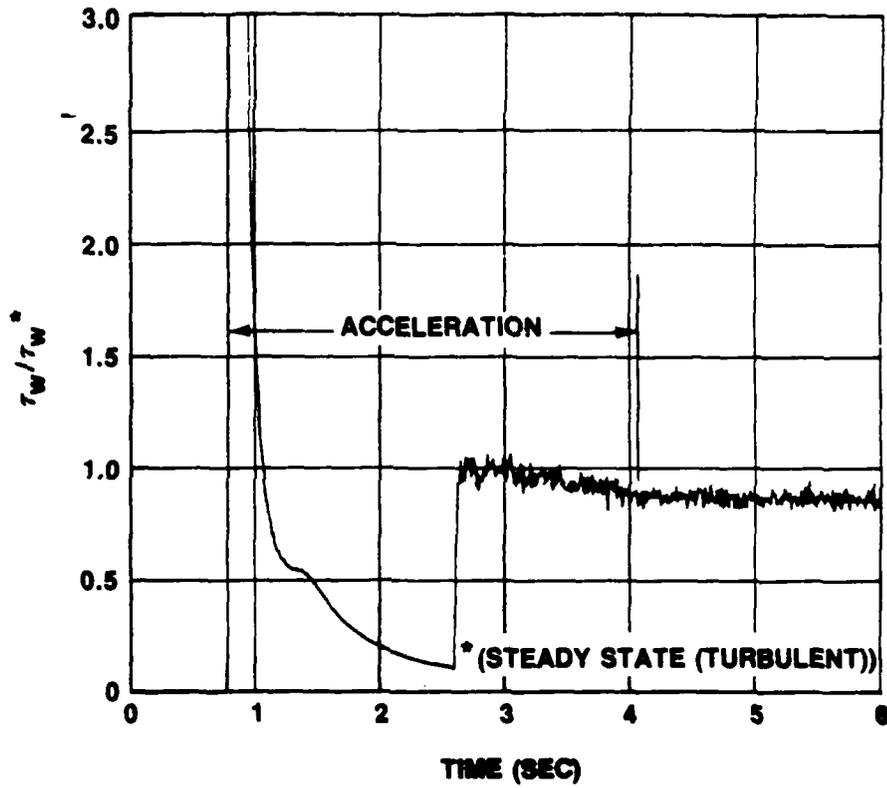
Figure IV-79.  $\tau_w$  Nondimensionalized by Quasi-Steady Turbulent Value at  $\ddot{X} = 2.4 \text{ m/s}^2$  and  $U_{m0} = 0$
