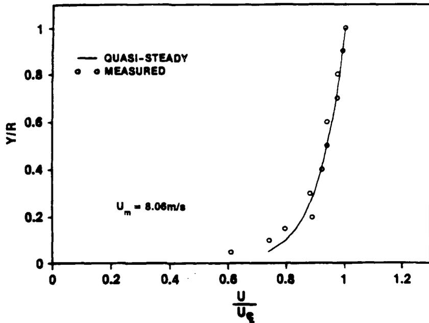
Figure 55o. Velocity Profile at  $t = 4.000$  s ( $t^* = 0.00455$ ) for  $\ddot{X} = 2.4$  m/s<sup>2</sup> and  $\bar{U}_{m0} = 0$
