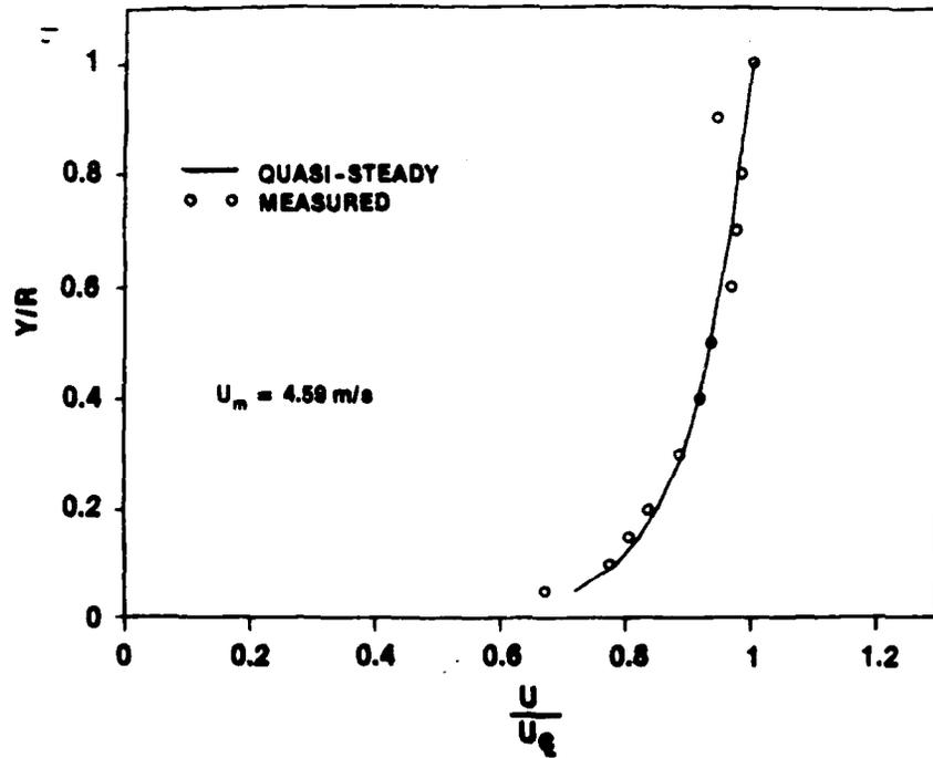
Figure 67g. Velocity Profile at  $t = 2.200$  s for  $\ddot{X} = 2.4$  m/s<sup>2</sup> and  $\bar{U}_{m0} = 1$  m/s
