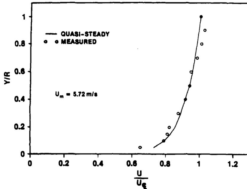
Figure IV-55m. Velocity Profile at  $t = 3.000$  s ( $t^* = 0.00323$ ) for  $\ddot{X} = 2.4$  m/s<sup>2</sup> and  $\bar{U}_{m0} = 0$
