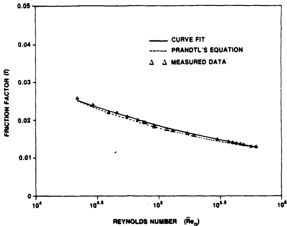
Figure II-6. Test Section Friction Factor vs Reynolds Number
