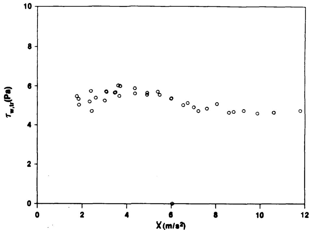
Figure IV-33. Wall Shear Stress vs Acceleration at Transition
