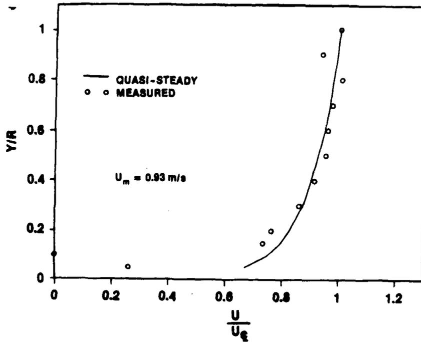
Figure 67a. Velocity Profile at  $t = 0.600$  s for  $\ddot{X} = 2.4$  m/s<sup>2</sup> and  $\bar{U}_{m0} = 1$  m/s
