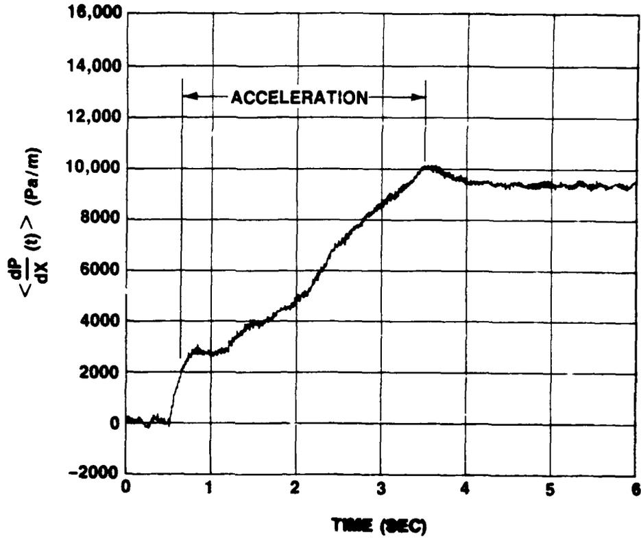
Figure IV-100.  $\langle dp/dx(t) \rangle$  vs  $t$  for Ensemble Average of 20 runs at  $\ddot{X} = 2.4 \text{ m/s}^2$  and  $\bar{U}_{m0} = 1 \text{ m/s}$
