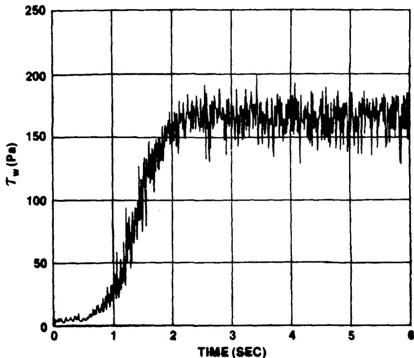
Figure IV-91.  $\tau_w$  vs  $t$  for One Typical Run at  $\bar{X} = 6.1 \text{ m/s}^2$  and  $\bar{U}_{m0} = 1 \text{ m/s}^2$
