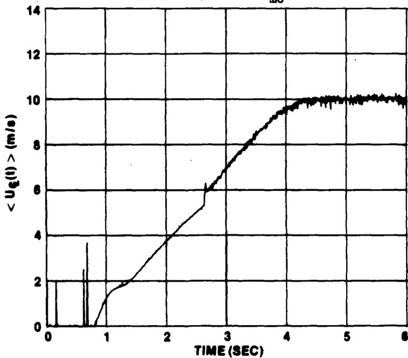
Figure IV-51.  $\langle U_{c1}(t) \rangle$  vs  $t$  for Ensemble Average of 20 Runs at  $\ddot{X} = 2.4 \text{ m/s}^2$  and  $\bar{U}_{m0} = 0$
