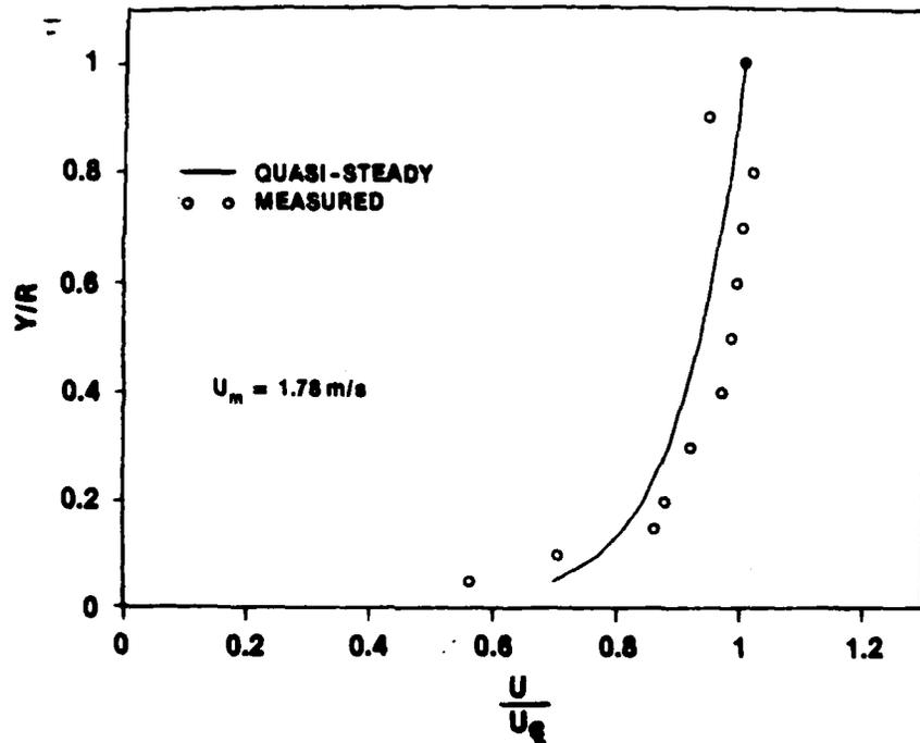
Figure 67c. Velocity Profile at  $t = 1.000$  s for  $\ddot{X} = 2.4$  m/s<sup>2</sup> and  $\bar{U}_{m0} = 1$  m/s
