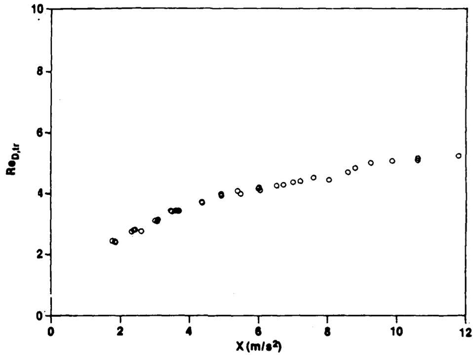
Figure IV-29. Pipe Reynolds Number vs Acceleration at Transition
