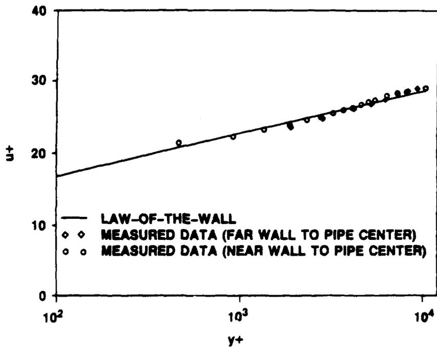
Figure IV-3. Steady-State Velocity Profile at  $Re_D = 450,000$
