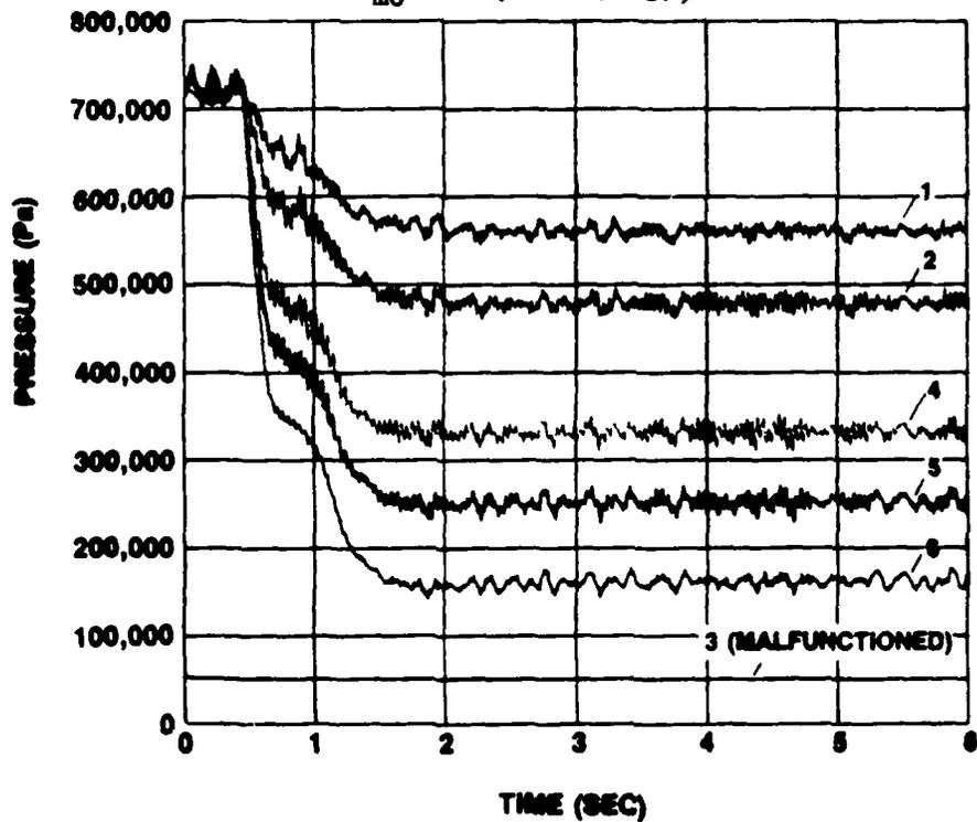
Figure IV-28. Pressure vs  $t$  for  $\ddot{X} = 11.79 \text{ m/s}^2$  and  $\bar{U}_{m0} = 0$  (Run No. 37)
