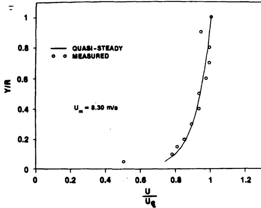
Figure 67k. Velocity Profile at  $t = 4.000$  s for  $\ddot{X} = 2.4$  m/s<sup>2</sup> and  $\bar{U}_{m0} = 1$  m/s
