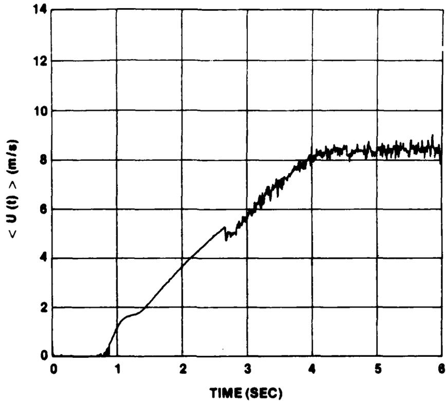
Figure IV-53.  $\langle U(t) \rangle$  at  $r/R = 0.80$  vs  $t$  for Ensemble Average of 20 Runs at  $\bar{X} = 2.4 \text{ m/s}^2$  and  $\bar{U}_{m0} = 0$
