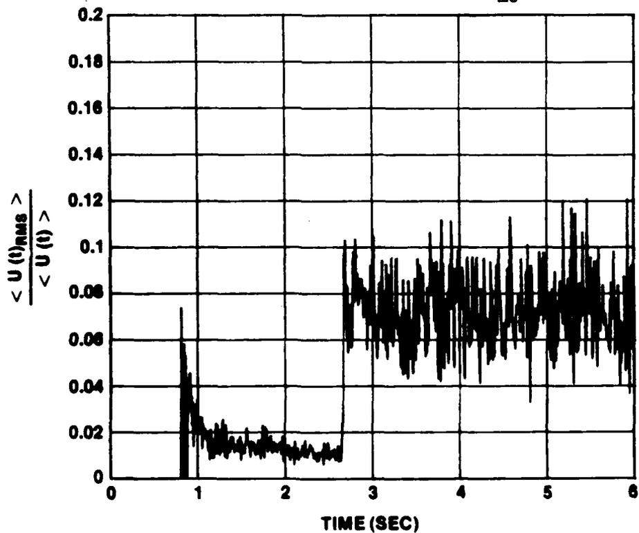
Figure IV-53. RMS of  $\langle U(t) \rangle$  at  $r/R = 0.80$  vs  $t$  for Ensemble Average of 20 Runs at  $\bar{X} = 2.4 \text{ m/s}^2$  and  $\bar{U}_{m0} = 0$
