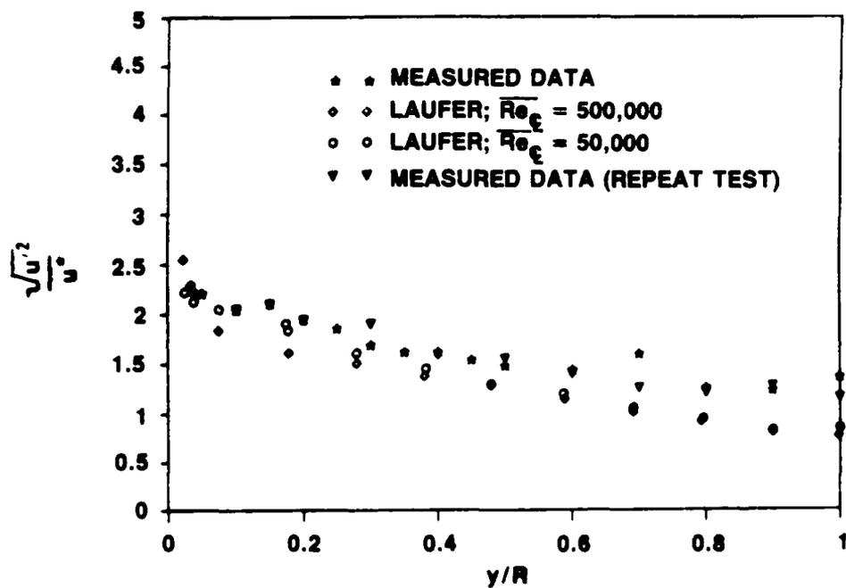
Figure IV-6. Steady-State Turbulence Intensity at  $\overline{Re}_D = 275,000$
