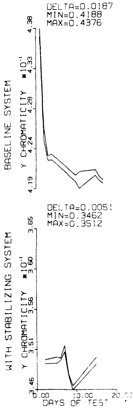
Figure 24. Comparison Using Conrac Monitor of Long-Term Drift in y CIE Chromaticity Coordinate Between Baseline and Compensated Display System.
