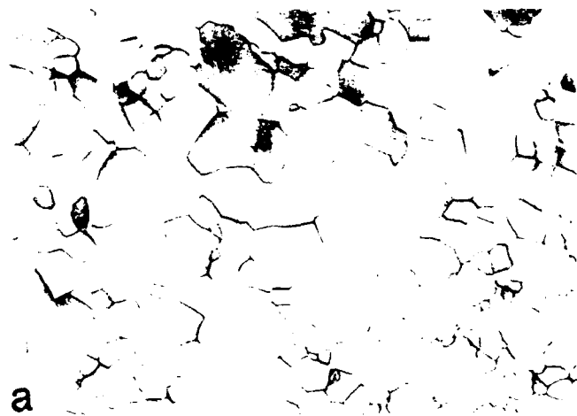
Figure 10. Microstructure of the Stoichiometric Ni-Al Alloy (Wt.-% Ni = 49.5) Cast from a VIM Ingot and Extruded at 1000°C with an Extrusion Ratio of 1.5. (a) Transverse Section, (b) Longitudinal Section.
