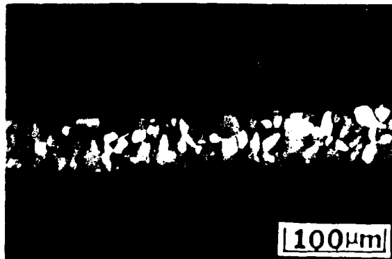
Figure 1. Micrographs of the surface of the Al 2 O 3 Nanoparticles (No. 24) after Al 2 O 3 Nanoparticles are mixed with the epoxy resin and cured. The surface of the epoxy resin is treated with the Al 2 O 3 Nanoparticles. After curing, the surface of the epoxy resin is shown.
