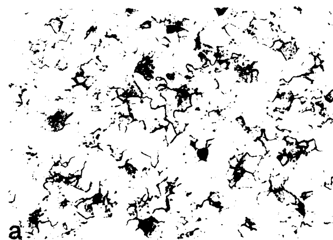
Figure 11. Microstructure of the Stoichiometric Ni-Al Alloy (Wt.-% Ni = 49.5) Cast from a VIM Ingot and Extruded at 1000°C with an Extrusion Ratio of 1.5 and then Aged at 600°C for 100 Hours. (a) Transverse Section, (b) Longitudinal Section.
