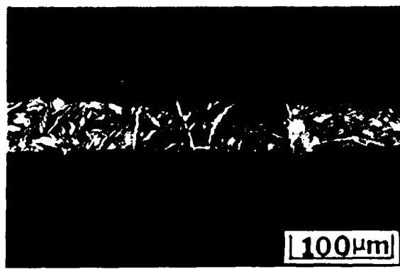
Figure 4. Microstructure of NiAl Alloy Number 86 (Ni-30.3 at% Al-30.3 at% Mn) prepared using a Melt Spinning Technique and in Various Heat Treatment Condition, (a) As-Solidified, After 2 hours at (b) 800°C, (c) 800°C and (d) 1200°C.
