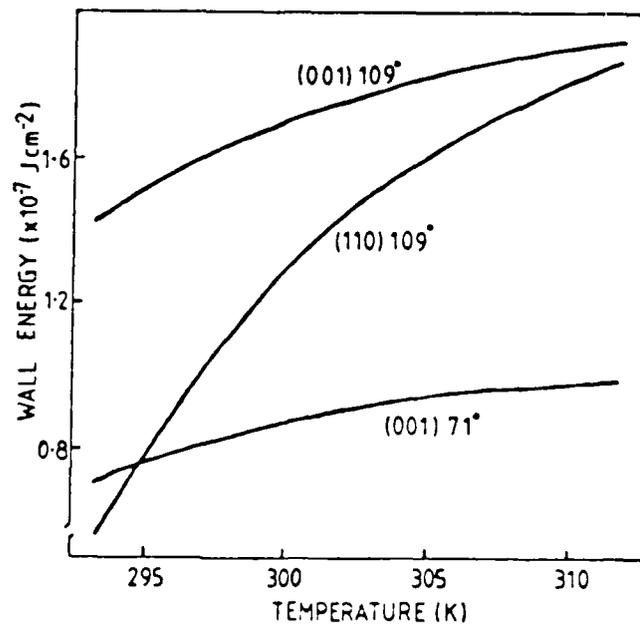
Fig.7: Energy of the indicated domain walls as a function of temperature (after ref.4).
