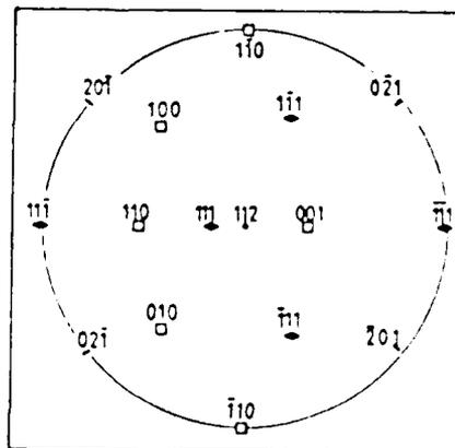
Fig.5: Orientation of various planes of (112) relative to  $\langle 110 \rangle$ .
