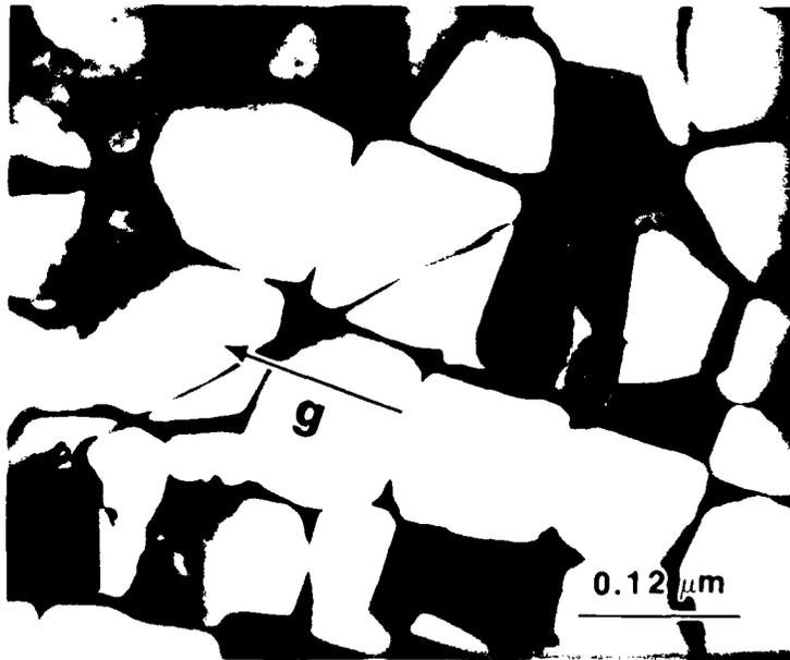
Figure 2.1-33 Dark field TEM image of sample L showing the "mace" type APBs in the  $\gamma'$  interior indicative of anisotropic APB energy associated with the system.
