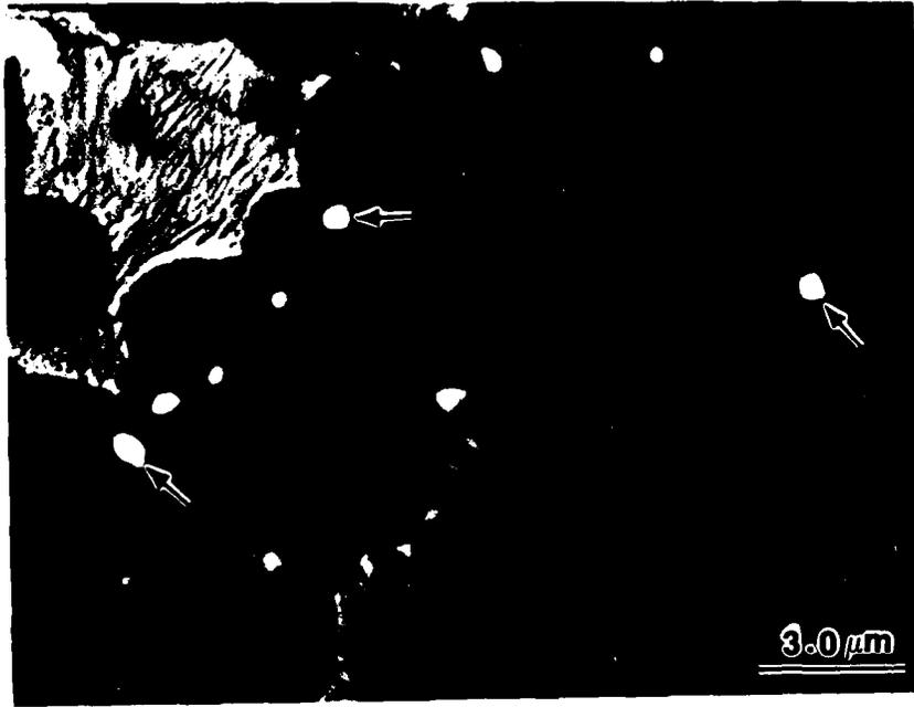
Figure 2.1-5 Scanning electron micrograph of sample J, showing dendrites, eutectic structure and partially dissolved hafnium particles as indicated by arrows.
