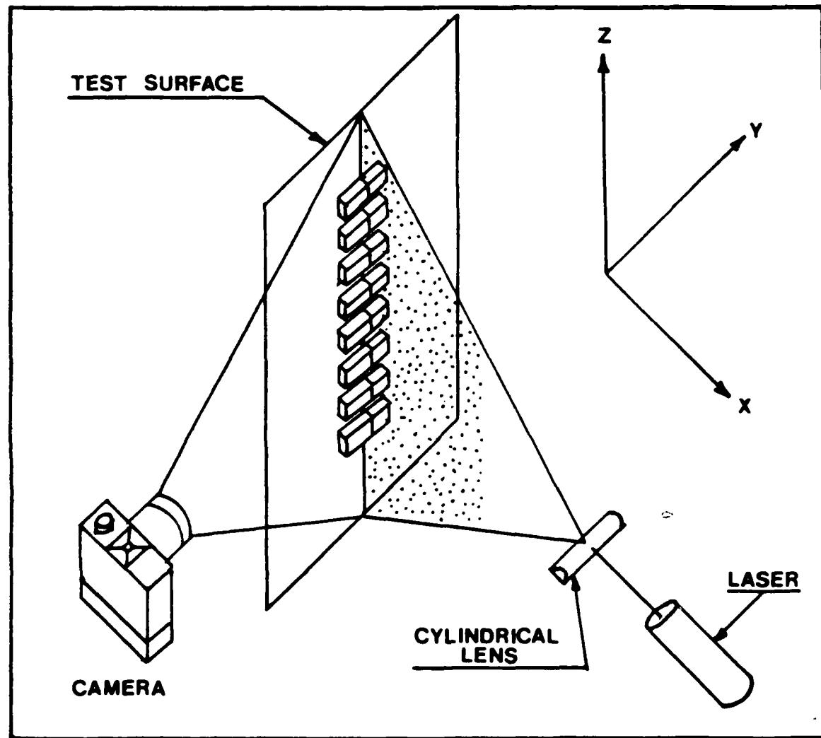
Figure 9. Laser and Camera Orientation
