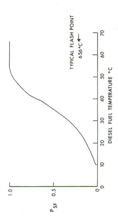
Probability of a Sustained Fire When an 81 mm (3.2 inch) Precision Shaped Charge is used to Attack Diesel Fuel in an Aluminum Test Fixture with Adequate Ventilation. Figure 1.
