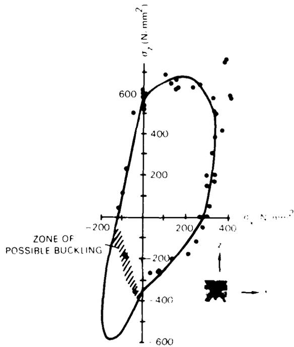
Figure 4-7. Biaxial fracture data of a  $[90/\pm 30/90]$  glass/epoxy laminate (Reference 16).
