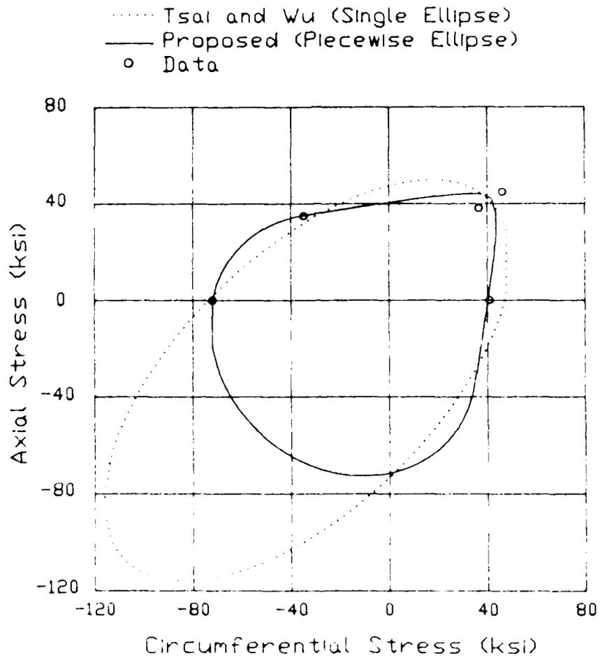
Figure 5-2 Correlations of the quadratic strength tensor theories with the biaxial fracture data of a (0/90/0/90)<sub>s</sub> graphite/epoxy laminate (Reference 13)
