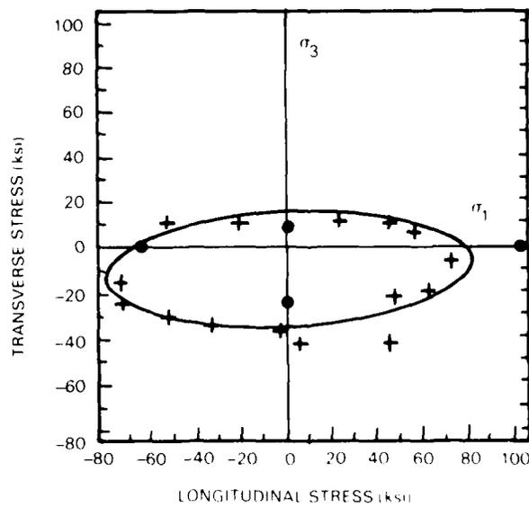
Figure 4-4. Biaxial fracture data of graphite/aluminum lamina (Reference 14).
