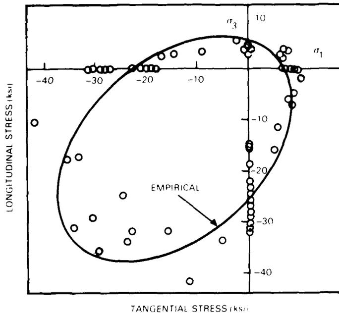
Figure 4-3. Biaxial fracture strengths for JT-50 composite material (Reference 9).
