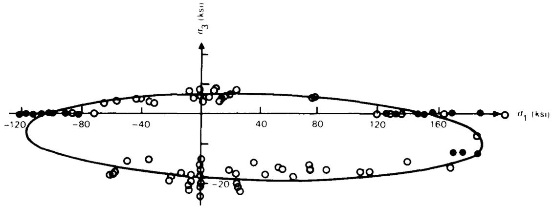
Figure 4-1. Biaxial fracture data of graphite/epoxy lamina (Morganite II) (Reference 13).
