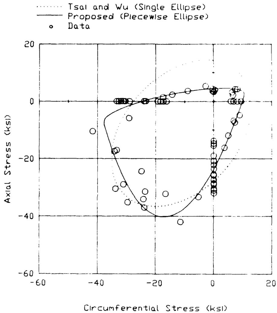
Figure 5-3 Correlations of the quadratic strength tensor theories with the biaxial fracture data of JT-50 composite material (Reference 9).
