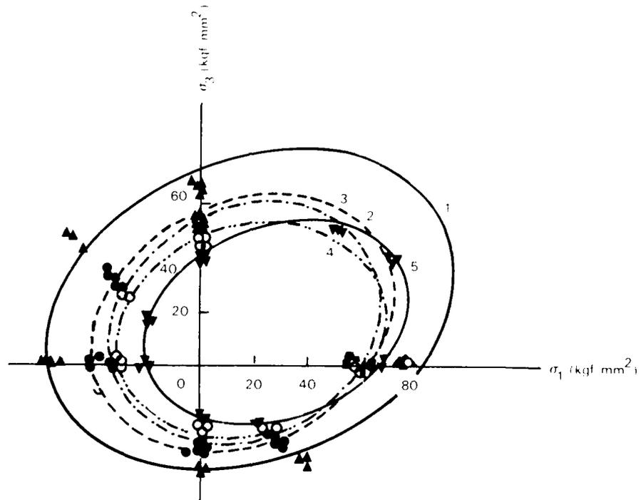
Figure 4-10. Biaxial fracture data for glass textolite (1), hybrid textolite with  $\mu' \text{ gf } \mu''$  of  $\approx 0.7 : 0.3$  (2),  $0.5 : 0.5$  (3),  $0.3 : 0.7$  (4), and organic textolite (5) (Reference 18).
