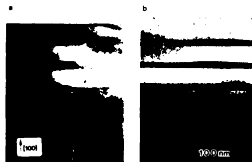
FIG 2 Cross-section TEM's of samples 284 (a) and 334 (b) showing commensurate growth. The SiGe layers appear darker in these micrographs. Plan view images show that the dislocation density is less than 10^6 \text{ cm}^{-2} (Hewlett-Packard Labs)
