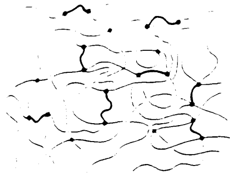
Figure 2. A network having a bimodal distribution of network chain lengths. 4 The very short polymer chains are arbitrarily represented by heavy lines and the relatively long chains by thinner lines.
