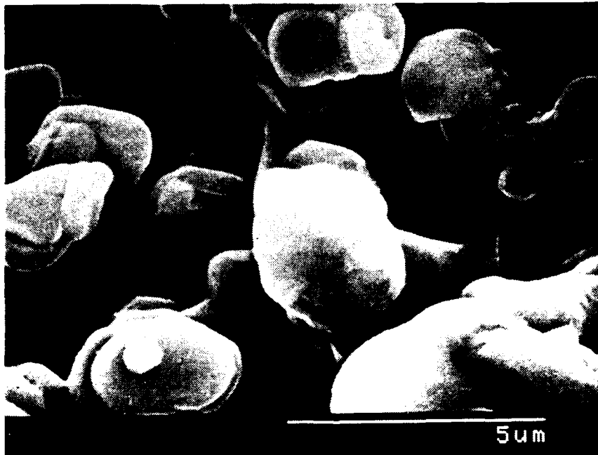
Figure 2.1A YBa 2 Cu 3 O 7-x Particles in Freeze-Dried Granule Calcined 16.5 hours at 900°C Batch 24729 10,000X
