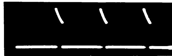
Fig 28. Influence of the Ribbon Across the Span of Model 6. Free Stream Velocity: 11.6 m/s; Input: 333 Hz at 3.75 V_{rms} ; x_r = 127 mm; y_r \approx 0 mm; x_a = 159 mm; y_a = 1 mm
