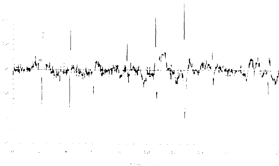
Figure 5-13. Elevator deflection (deg). Fixed gain control law. Plant parameter change and sensor noise. (std. dev. = 0.0573 deg (deg/sec))
