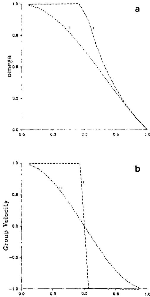
Fig. 1: The computational frequency (a) and computational group velocity (b) of the explicit scheme normalized by the analytical exact value. The abscissa represents the variable  $\kappa\Delta x$  normalized by  $\pi$ . (I)  $\tau = 0.01$ , or  $\Delta t = 1.75$ ; (II)  $\tau = 0.5$  or  $\Delta t = 87$ .
