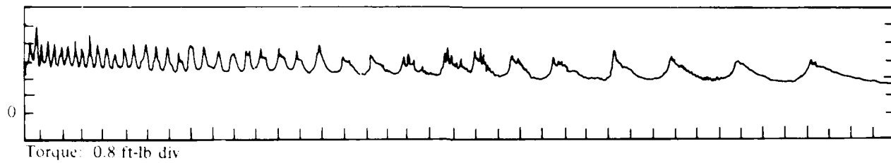
Figure 16. Dynamometer recording showing torque data. Chart speed 1 mm/sec.
