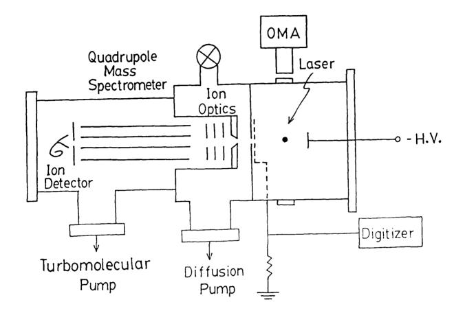
Fig. 1. Schematic diagram for the apparatus constructed for analyzing the chemical species in discharge media.
