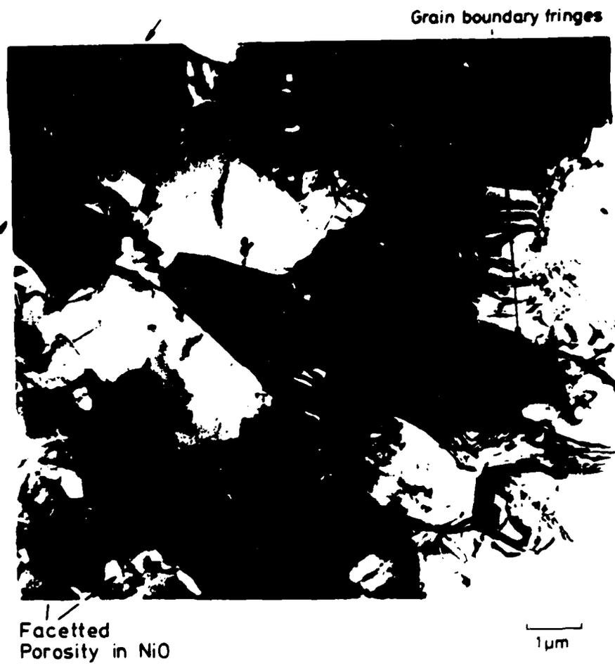
Fig. 11. Transverse TEM Micrograph of Scale Grown on Ni at 800°C for 21 hours (Specimen 58)
